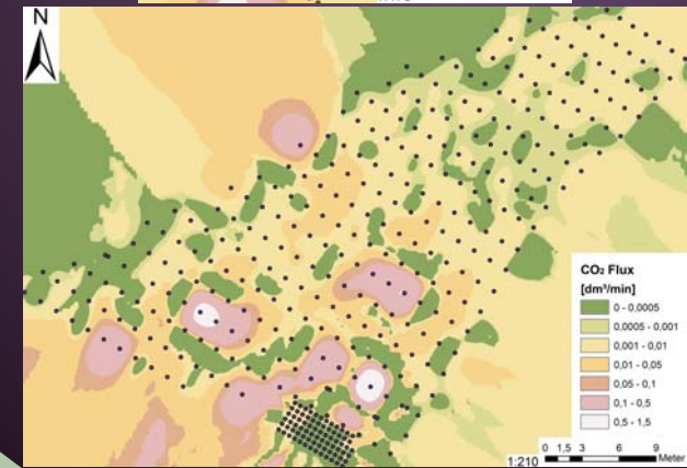
Fig.4: Position of flux measurements and interpolation of CO 2 flux.
