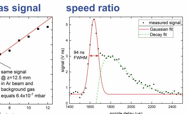
measured ion pulses generated by laser induced photoelectrons in ionization volume!
