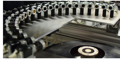
Fig. 2. The tomography setup around the swirl burner, showing 24 cameras with filters arranged around the burner.
