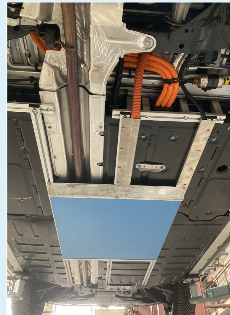
Figure 2 - 22 kW wireless charging vehicle coil installed under the battery
