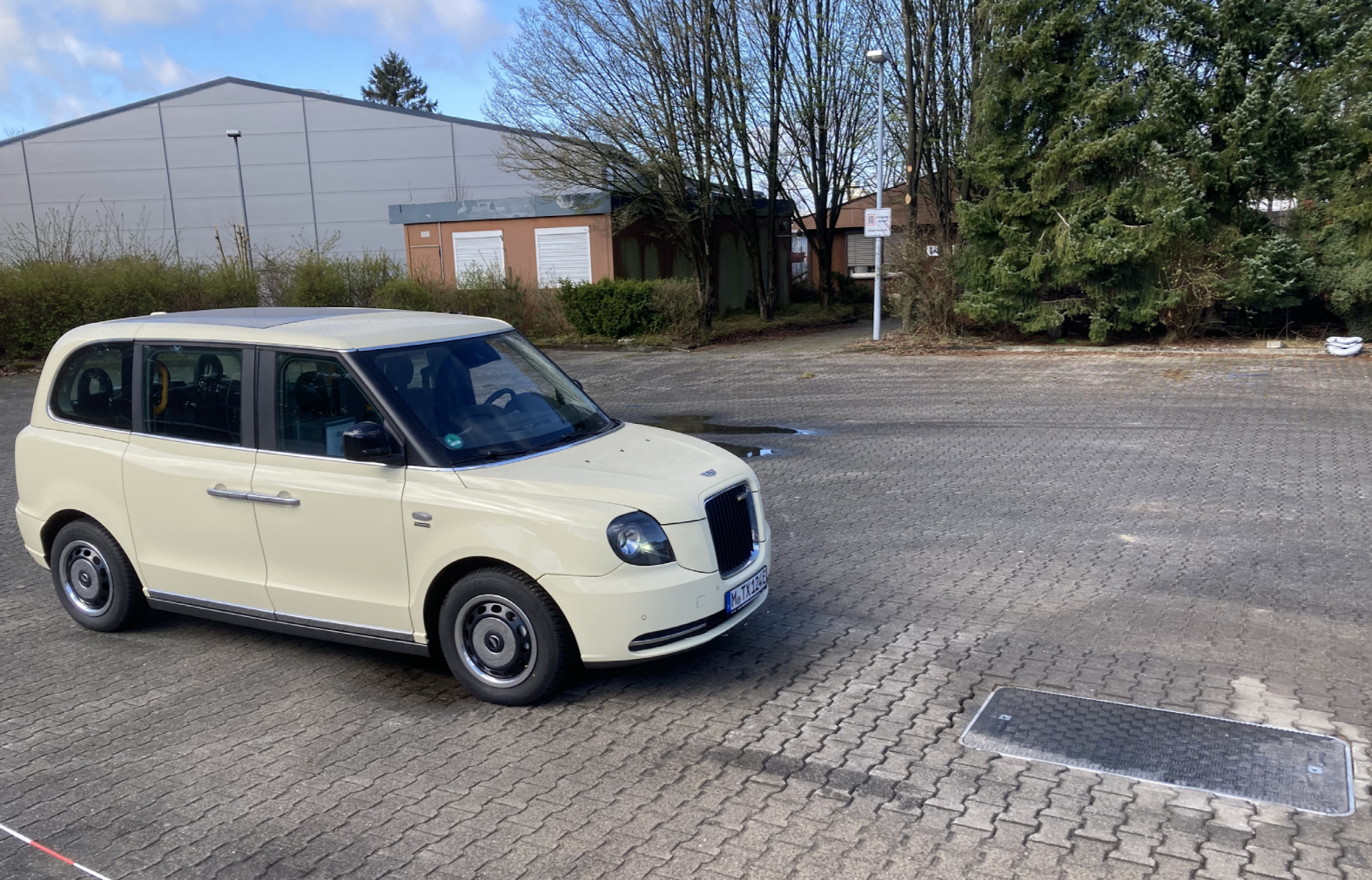
Figure 3 - LEVC TX and 22 kW wireless charging installation at INTIS' test centre Germany
