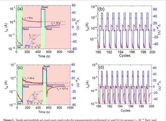
Figure 5. Single and multiple set-read-reset-read cycles for measurements performed (a) and (b) in vacuum ( $\sim 10^{-6}$  Torr) and under  $N_2$  atmosphere at a pressure of 760 Torr (c) and (d).
