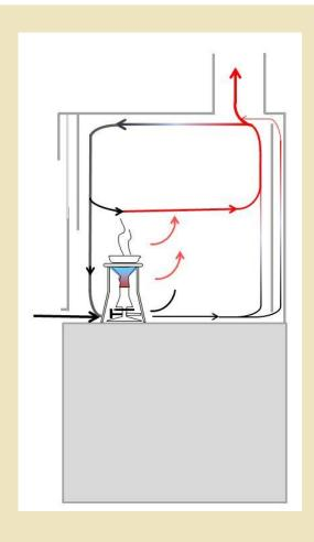
Set-up heating apparatuses at the back of the fume hood!
