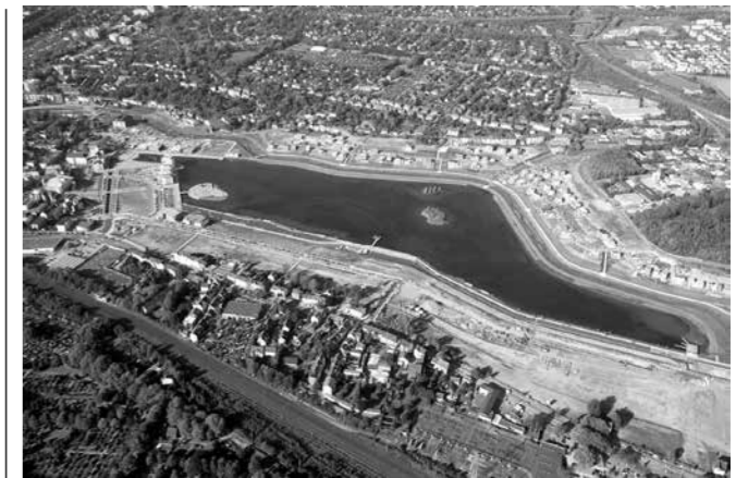
(1) Phoenix Lake in Dortmund, Germany. The lake is an example of urban integrated watershed management, where the area, a former industrial plant, was revitalized featuring a lake for flood retention, recreational and commercial areas, as well as housing. Source: Rupert Oberhäuser/Emschergenossenschaft
