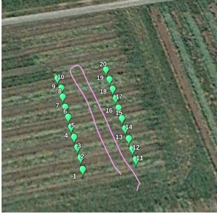
Fig. 4. Flight trajectory (purple) during the experiment with GPS-RTK reference positions for terrain measurement (green dots)
