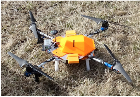
Fig. 2. Drone for measurements, all distance sensors are directed downward.
