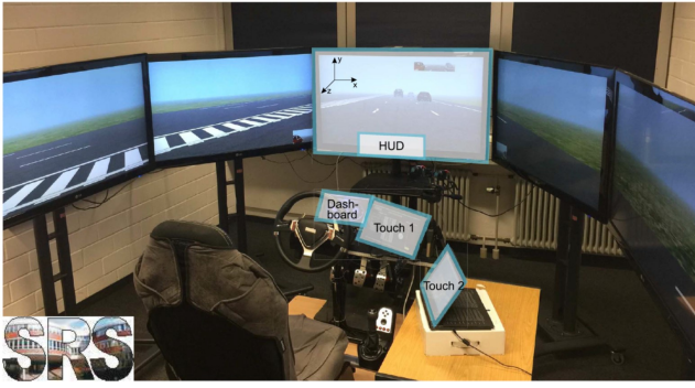
Fig. 2. Driving simulator laboratory, Chair of Dynamics and Control, U DuE
