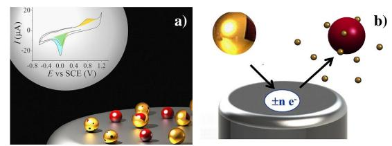
**Figure 1.** Schematic drawing of (a) nanoparticle ensemble studies of core-shell nanoparticles and (b) single nano-impact studies.
