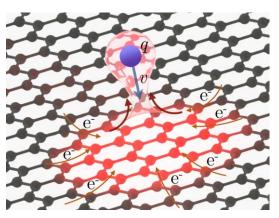
We take the final step and transmit slow (< 1 a.u.) highly charged Xe ions with charge states (q > 30) far away from equilibrium through the ultimately thin 2D material, a freestanding single layer of graphene.
