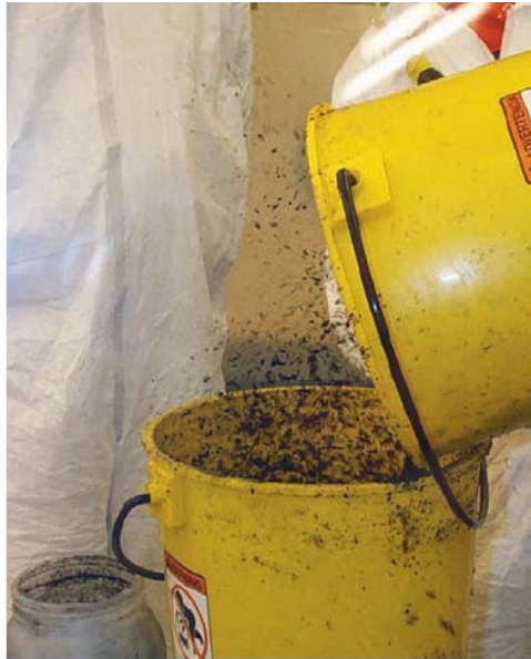
Figure 8. Pouring HiPCO ® nanotube material between containers at Rice University
