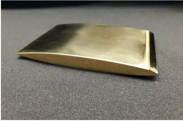
Figure 1. The photo of the benchmark hydrofoil CAV2003 with a miniature wedge-type vortex generator on the suction side of the hydrofoil.
