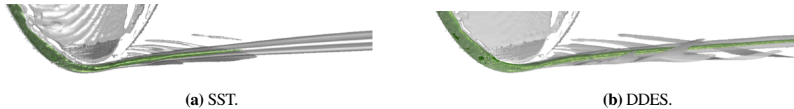
Figure 12: Vortical flow near the tip as viewed from the suction side with different turbulence modelling. EE simulations on the fine grid. Visualization with Q=5 \times 10^4 based on volumetric mixture velocity.
