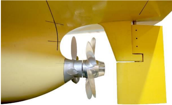
Fig.2 Hull model appended for self-propulsion test
