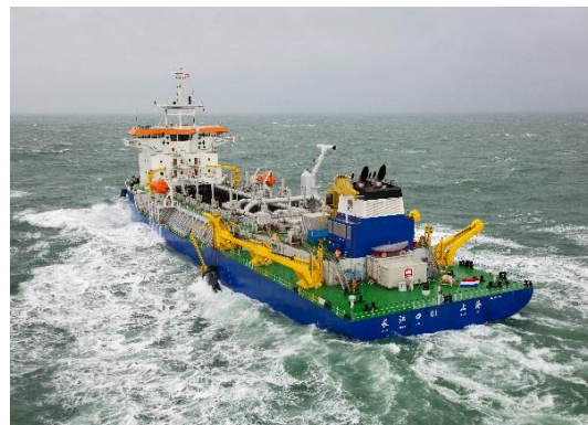
Fig. 2: Example of TSHD in dredging condition.
