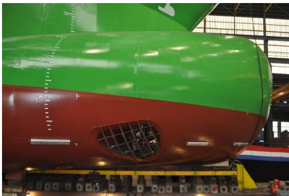
Fig. 1: Example of wing shaped cross section for bow thruster tunnel.
