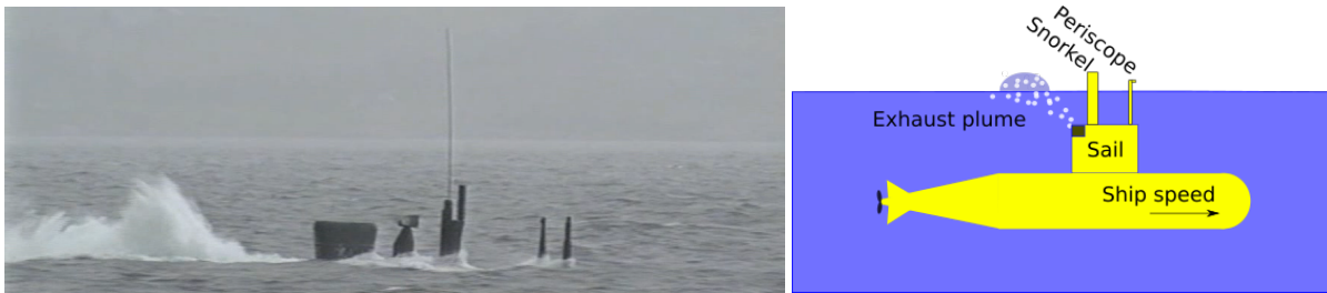
(a) Photograph of the sea trial of a Walrus class submarine. The snorkel is the left most mast, on the left of that the surface elevation is visible, Ministerie van Defensie (1990)
