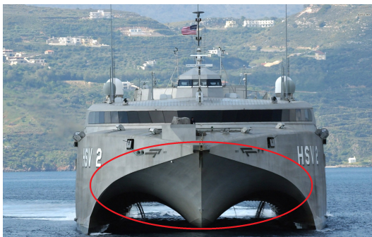
(b) The naval HSV catamaran with wave piercing bows and a wedge shaped wetdeck to mitigate slamming loads.
