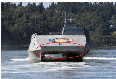
(a) X-craft naval catamaran showing the design of a flat wetdeck circled in red.
