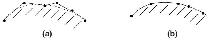
Fig. 2: Discretization of a curved geometry. (a) Finite element nodes do not exactly describe the surface whereas (b) the NURBS geometry exactly covers the surface. The figure is adapted from Hughes et al. (2005).
