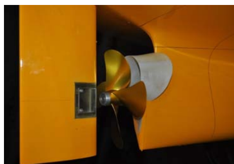
Fig. 5: The hull and the duct model.
