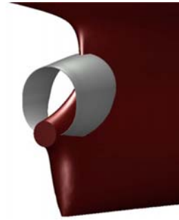
Fig. 2(b): The geometry of the optimized duct
