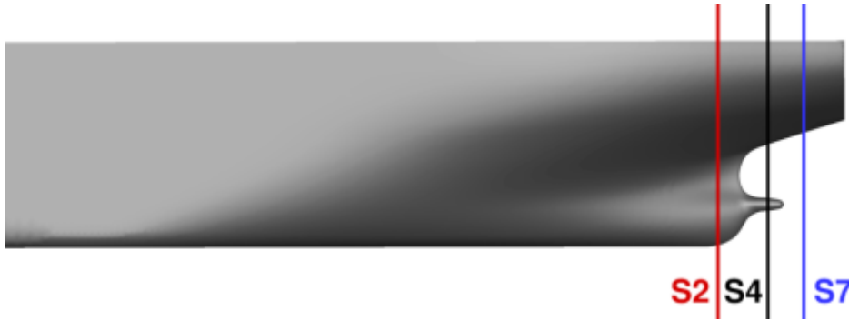
Fig. 2: Side view of the JBC hull with location of three measurement sections
