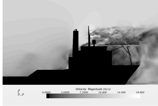
Figure 8: Velocity Magnitude from URANS (left) and DES (right) above the helideck
