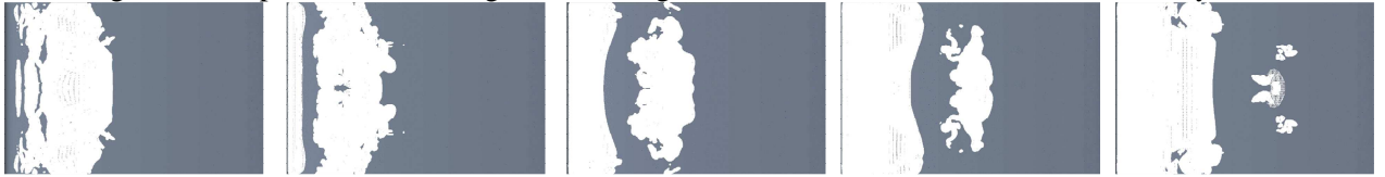
Fig. 12. CFD prediction. Scaling factor of negative cavitation rate 1. Seed nuclei density 10^{12} .
