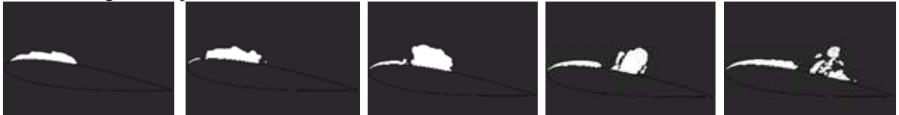
Fig. 15. CFD prediction. Scaling factor of negative cavitation rate 1. Seed nuclei density 10^{14} .
