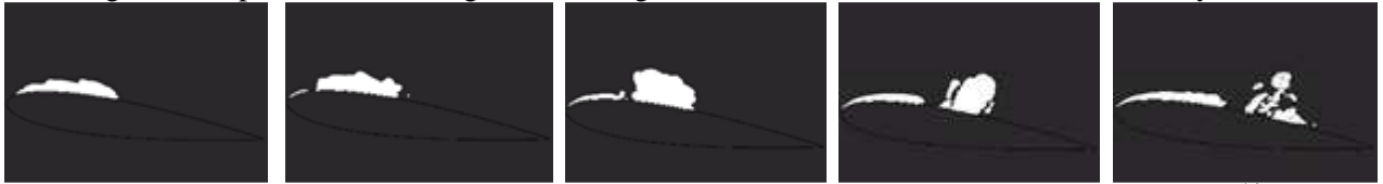
Fig. 8. CFD prediction. Scaling factor of negative cavitation rate 1. Seed nuclei density 10^{14} .
