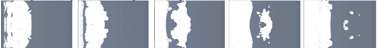
Fig. 13. CFD prediction. Scaling factor of negative cavitation rate 1. Seed nuclei density 10^{10} .
