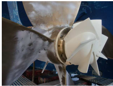
Fig.1 ECO-Cap attached to the actual ship
