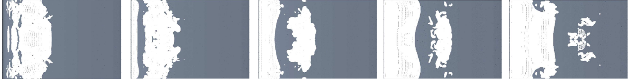
Fig. 11. CFD prediction. Scaling factor of negative cavitation rate 1. Seed nuclei density 10^{14} .
