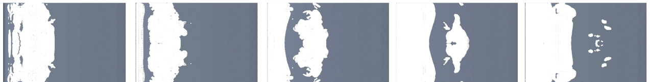
Fig. 3. CFD prediction. Scaling factor of negative cavitation rate 0.1. Seed nuclei density 10^{14} .
