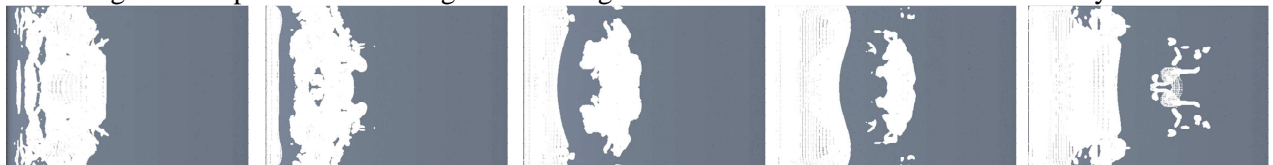
Fig. 5. CFD prediction. Scaling factor of negative cavitation rate 2. Seed nuclei density 10^{14} .
