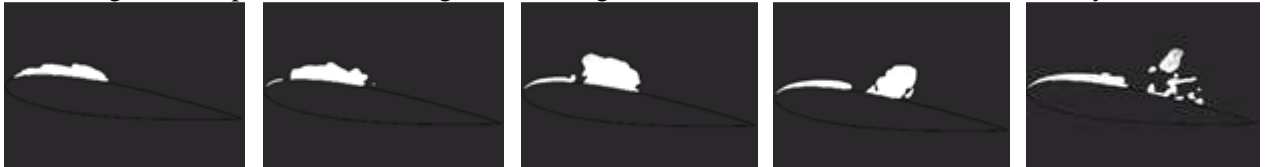
Fig. 9. CFD prediction. Scaling factor of negative cavitation rate 2. Seed nuclei density 10^{14} .
