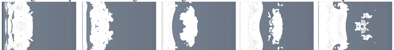
Fig. 4. CFD prediction. Scaling factor of negative cavitation rate 1. Seed nuclei density 10^{14} .
