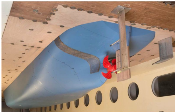
Figure 1 Hydrophone setup for noise measurement
