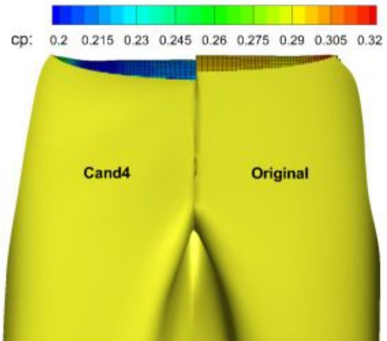
Figure 11 Pressure coefficient at the wetted part of the transom. Note that the range for the pressure only includes positive values.
