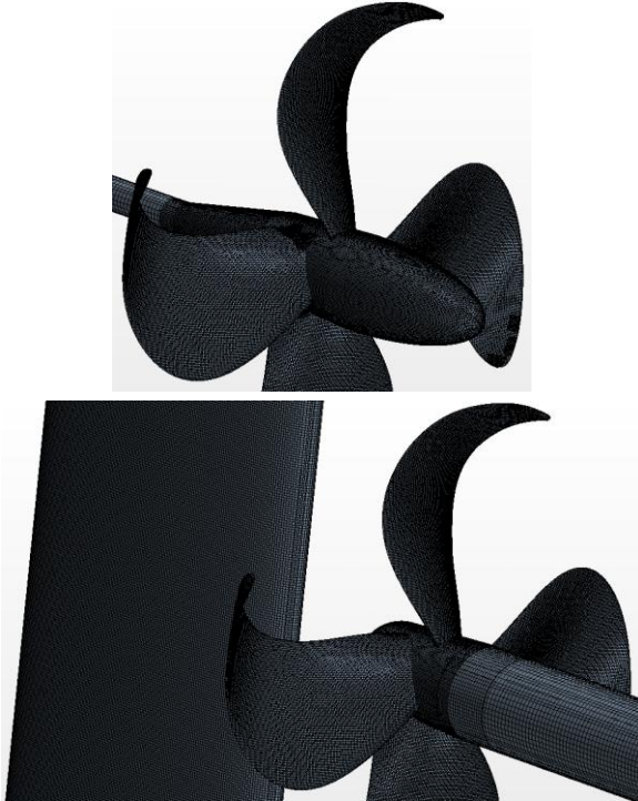
Fig. 2: Propeller surface mesh in the open-water simulation (top) and the simulation with the wake field and rudder (bottom)
