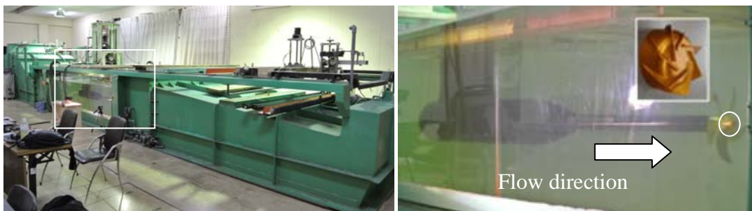
Fig.12 Measurement Equipments for the Propeller Characteristics by Reverse POT
