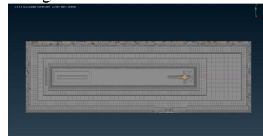
Figure 3: The coarse mesh for the open water test
