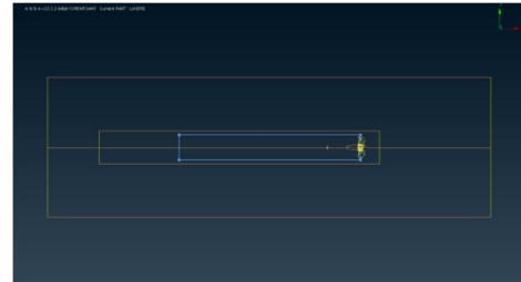
Figure 2: The propeller inside the MRF-zone (small region with thin line), the domain (large region with thin line) and size box (thick line)
