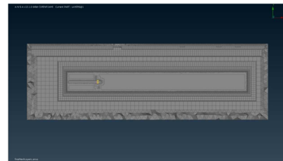
Figure 10: The fine mesh used for the velocity field measurement prediction
