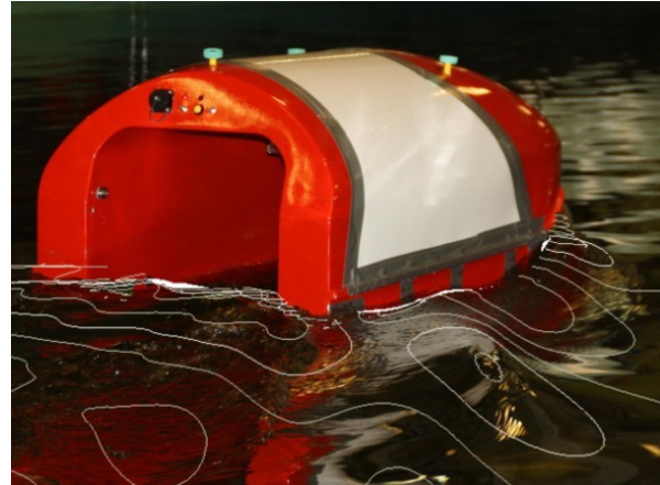
Figure 13: Superposition of simulated free-surface contour and image of free surface for free sailing AGAPAS catamaran model with s/L = 0.45 at \beta = 0^\circ and Fn = 0.4 .
