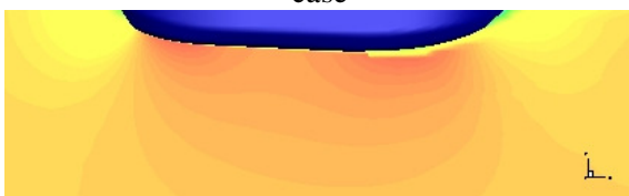
Fig. 11 Streamwise velocity contours in the propeller axis plane ( y=2.743 ) for hull with skeg case
