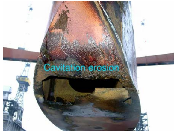
Fig.2: Rudder sole cavitation, GL photo
