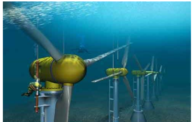
Fig. 1. A typical horizontal axis free stream marine current turbine.
