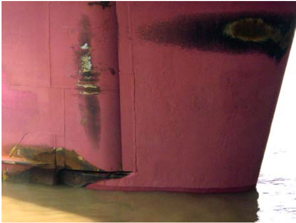
Fig.6: Gap cavitation, GL photo
