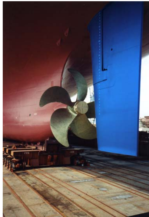
Fig.17: Special soft surface coating, GL photo
