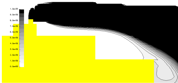
a) Funnel 5 m height without radar mast
