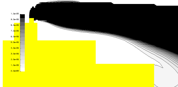
d) Funnel 7,5 m height with radar mast
