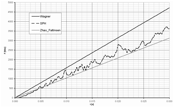
Figure 3: Time history of Normal Force on half-wedge, comparison of SPH with theoretical methods
