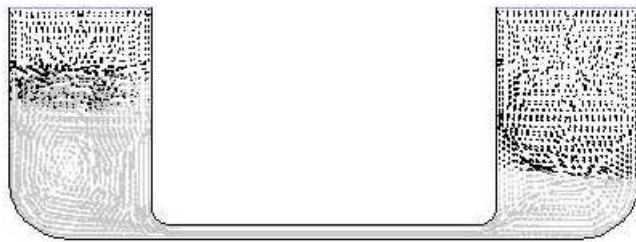
Figure 6. Rounding the U-tank angles
