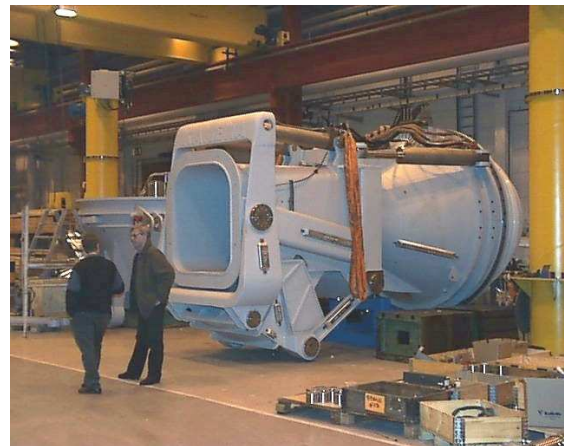
Fig. 2 Kamewa Waterjets Size 200 steering and reversing unit
