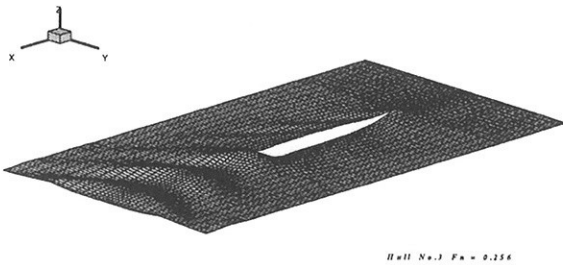
Fig. 15 Free surface elevation. Hull No.3 non-linear computation
