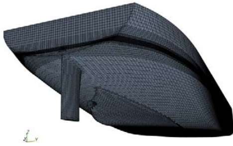
Figure 4: Computational grid on hull.
