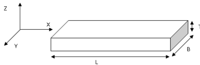
Fig.8: Barge: L=1.05 m, B=0.29 m, T = 0.025 m, C_B = 1 , mass = 7.26 kg, I_{yy}=0.7 kgm 2 , KG=0.025 m
