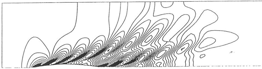
Figure 2. Overhead view of wave elevation (or pressure) contours for F_n=0.289 .
