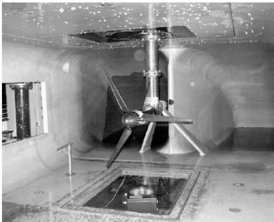
Figure 6. Photograph of the assembled test rig in the cavitation tunnel.
