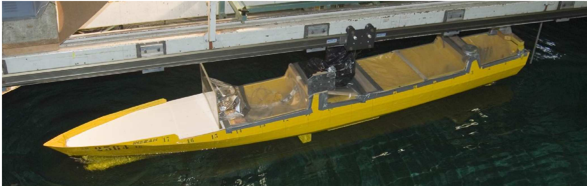
Figure 1: 3D experiments on a patrol ship model: global view of the model and deck set-up.
