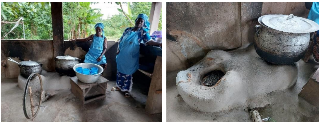
Fig. 22 and 23: Clay-built kiln fired with oil palm kernel shells, where the air supply is regulated by means of a manually operated flywheel.
