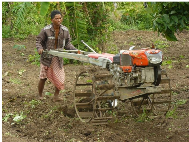
Photo 4: Hand-operated tractor, as it is used in many small farmers' households – a multifunctional device, which is also used as a traction "machine" for carts.
