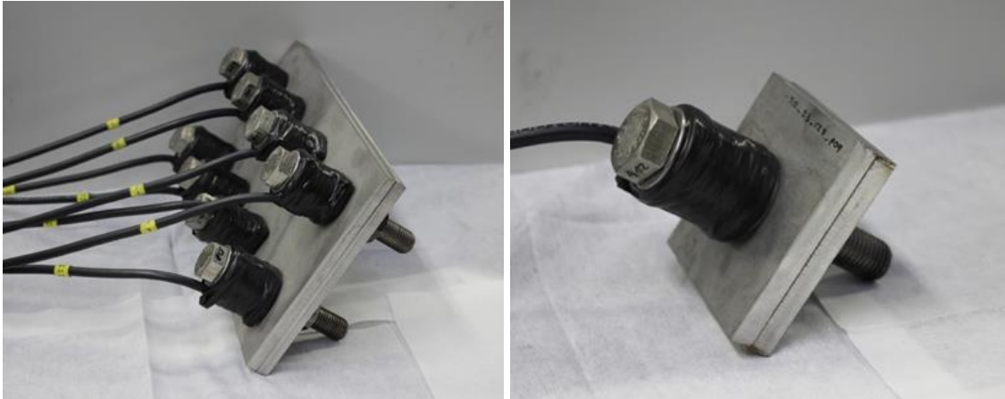
(a) Eight-bolt specimen (150 x 150 mm plate) (b) Single-bolt specimen (75 x 75 mm plate)
