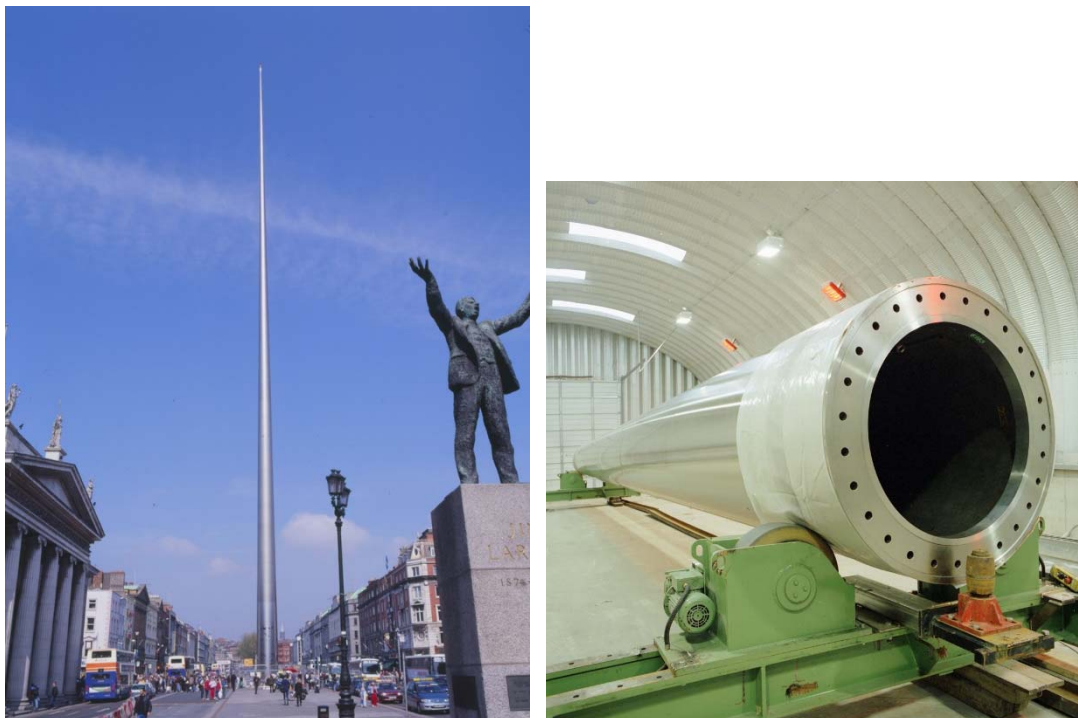
Figure 1.2 Spire of Dublin (left) and bolt holes in flange connection for a section of the Spire (right) (Photo: Norton Associates)
