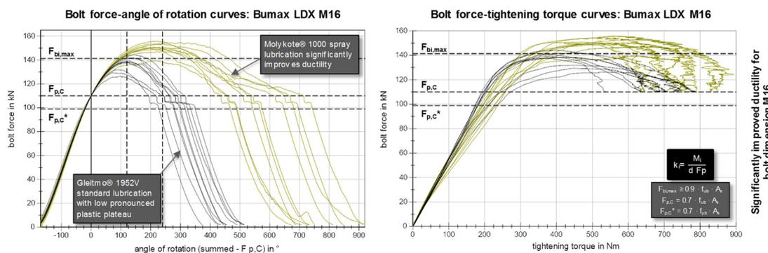
**Figure 112** Comparison of BU\_M16\_LDX tightening curves between gleitmo 1952V standard lubrication (black curves) and Molykote 1000 spray (yellow curves)
