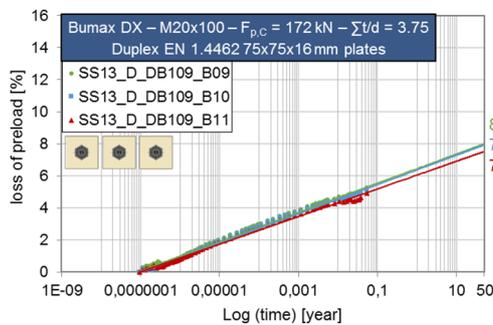
(a) preload losses-log (time) diagrams for one-bolt specimens
