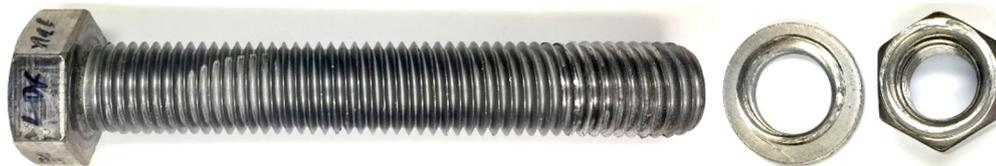
**Figure 46** BU\_M20\_LDX test specimen after tightening
