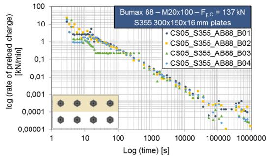
(b) log (rate of loss of preload) – log (time) diagrams for eight-bolts specimens - first row
