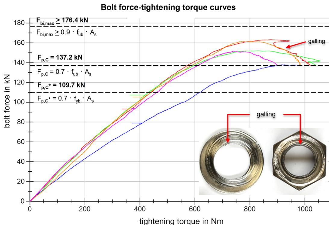
**Figure 39** BU\_M20\_88 (2013) Bolt force-tightening torque-curves
