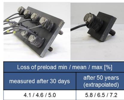
(d) loss preload measured/extrapolated after 30 days/ 50 years
