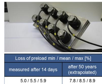
(c) loss preload measured/extrapolated after 14 days/ 50 years
