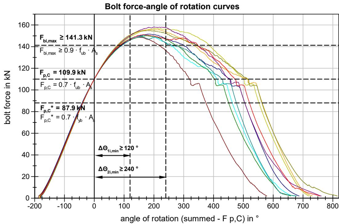
Figure 86 BU\_M16\_109 Bolt force-angle of rotation curves
