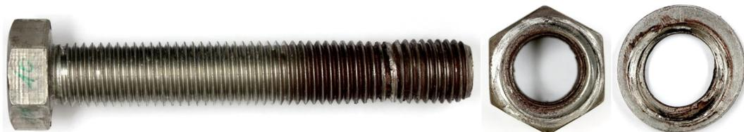
**Figure 85** BU\_M16\_109 test specimen after tightening
