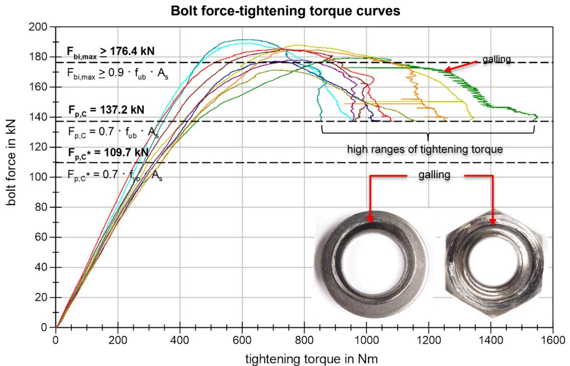
**Figure 42** BU\_M20\_88 (2015) Bolt force-tightening torque curves
