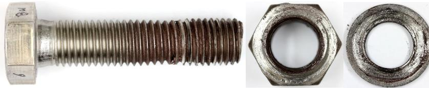
**Figure 58** BU\_M20\_88 (Molykote 1000 spray) test specimen after tightening
