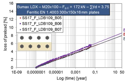
(b) preload losses-log (time) diagrams for eight-bolts specimens - second row
