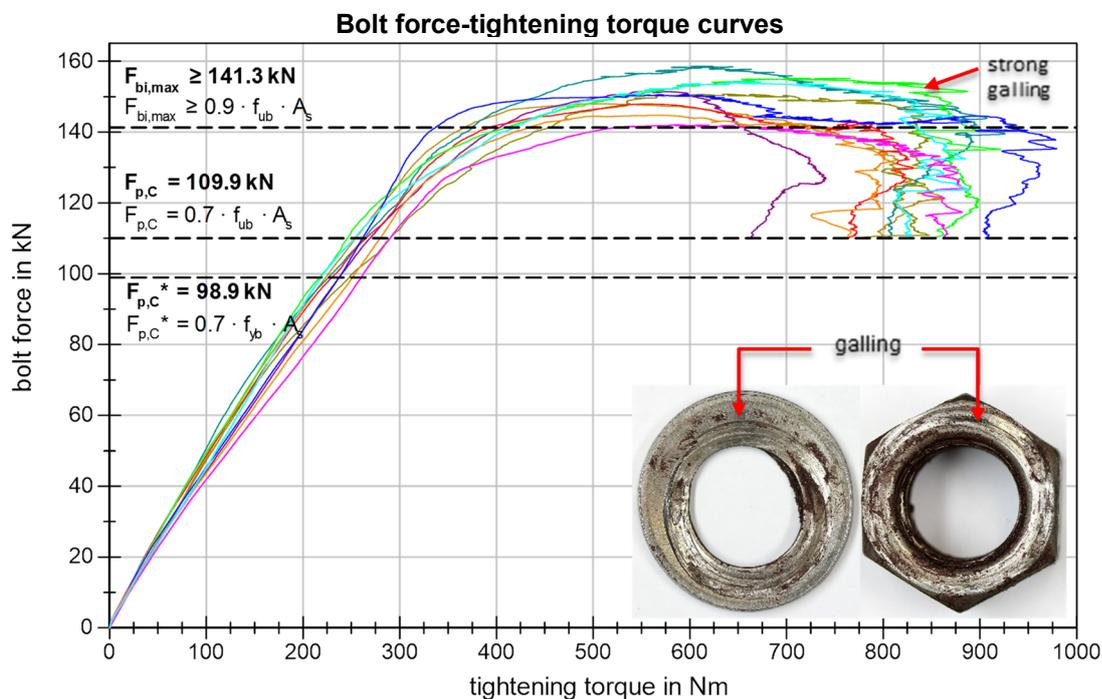
**Figure 96** BU\_M16\_DX Bolt force-tightening torque curves
