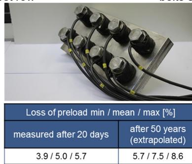
(c) loss preload measured/extrapolated after 20 days/ 50 years
