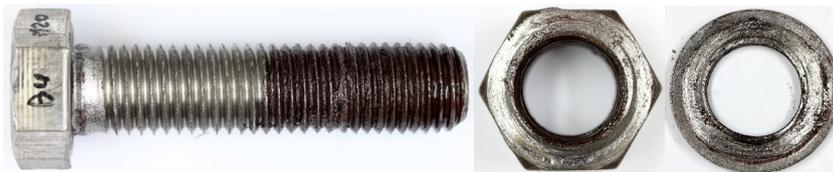
**Figure 61** BU\_M20\_88 (Molykote 1000 paste) test specimen after tightening
