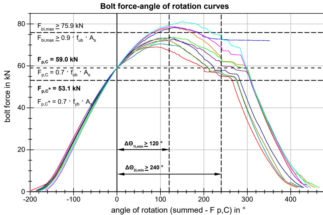
Figure 20 BU\_M12\_109 Bolt force-angle of rotation curves
