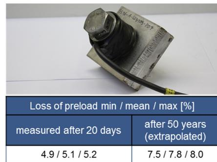
(b) loss preload measured/extrapolated after 20 days/ 50 years
