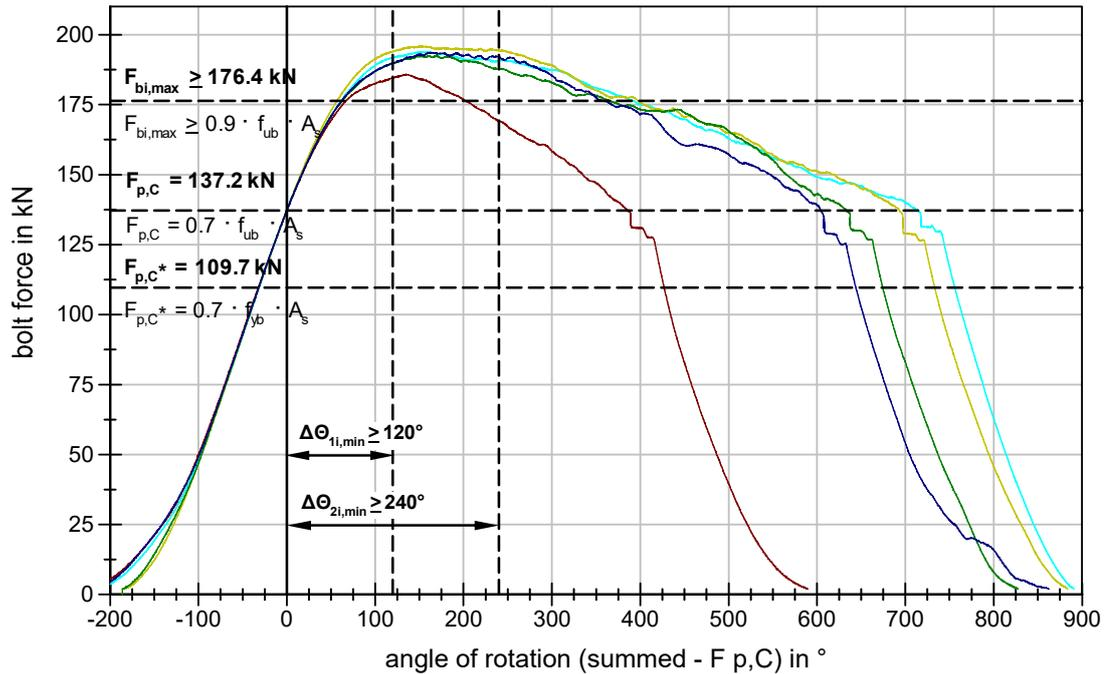
**Figure 59** BU\_M20\_88 (Molykote 1000 spray) Bolt force-angle of rotation curves
