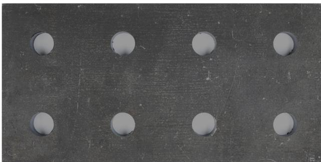
(c) Eight-bolts carbon steel specimens in 1D surface condition
