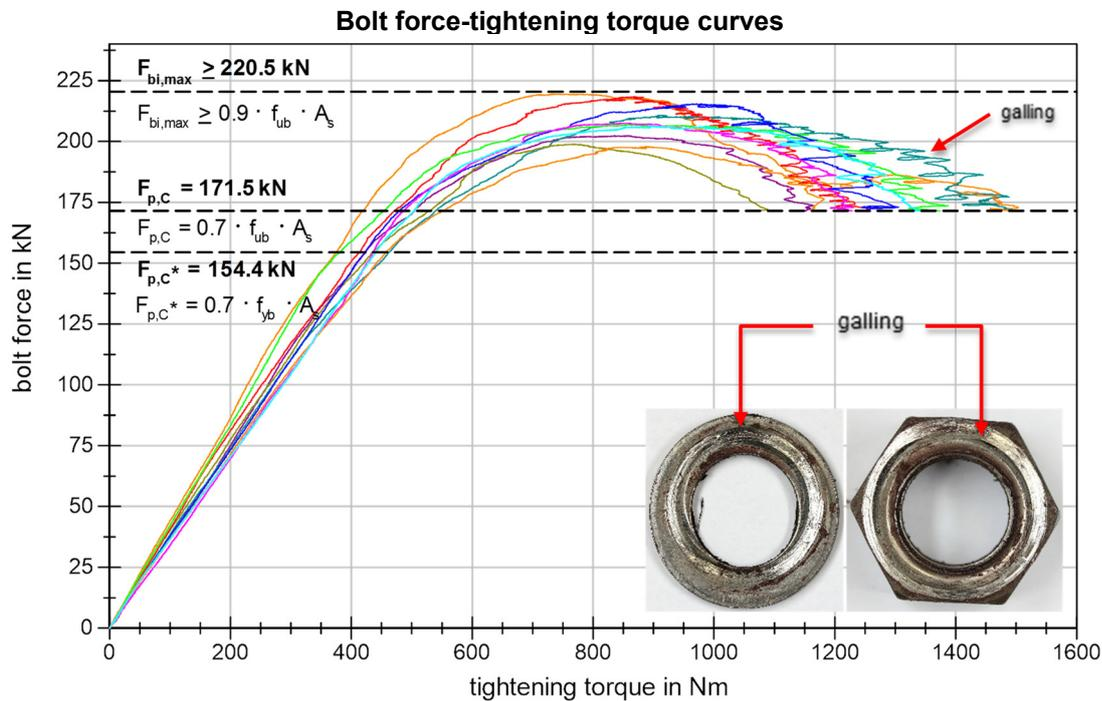
**Figure 78** BU\_M20\_LDX Bolt force-tightening torque curves
