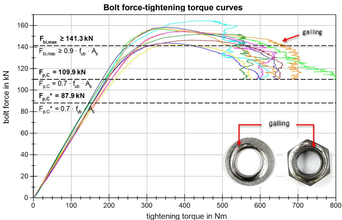
**Figure 90** BU\_M16\_109 Bolt force-tightening torque curves
