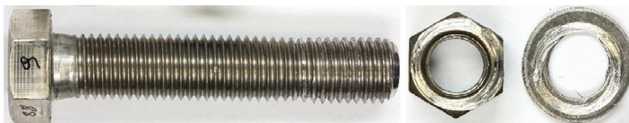
**Figure 40** BU\_M20\_88 (2015) test specimen after tightening
