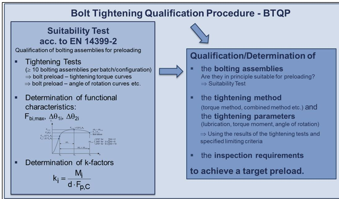
**Figure 118** Flowchart for suitability test and tightening method qualification of stainless steel bolts for preloading
