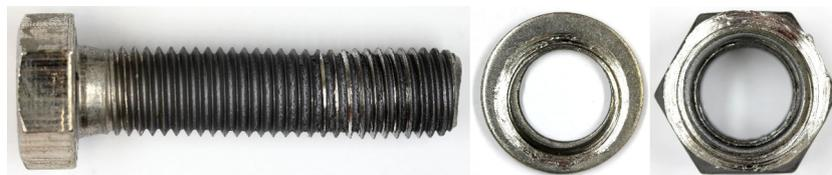
**Figure 67** BU\_M20\_88 (Molykote D-321R spray) test specimen after tightening
