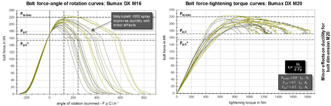
**Figure 113** Comparison of BU\_M20\_DX tightening curves between gleitmo® 1952V standard lubrication (black curves) and Molykote® 1000 spray (yellow curves)
