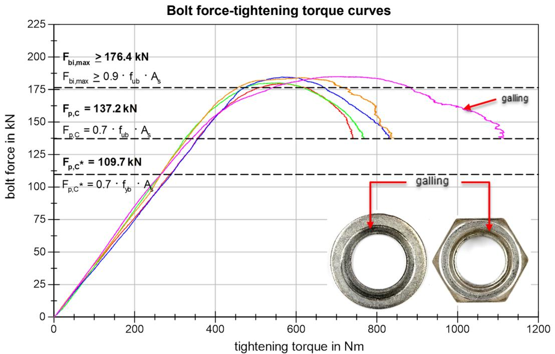
**Figure 57** BU\_M20\_88 (Gleitmo 1952V) Bolt force-tightening torque curves
