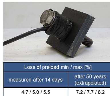
(b) loss preload measured/extrapolated after 14 days/ 50 years
