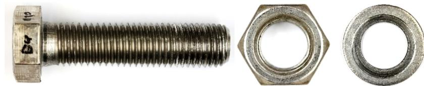
**Figure 55** BU\_M20\_88 (Gleitmo 1952V) test specimen after tightening
