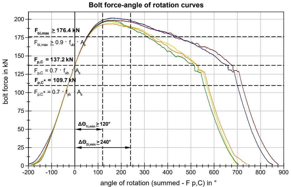
**Figure 68** BU\_M20\_88 (Molykote D-321R spray) Bolt force-angle of rotation curves
