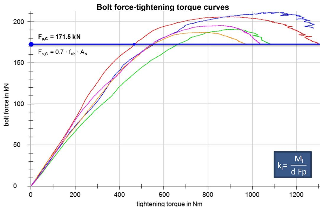
**Figure 99** BU\_M20\_LDX Bolt force-tightening torque curves – Interflon HT1200 spray
