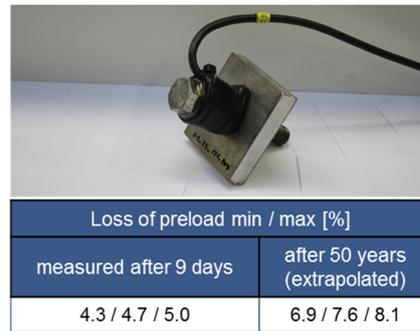
(b) loss preload measured/extrapolated after 9 days/ 50 years
