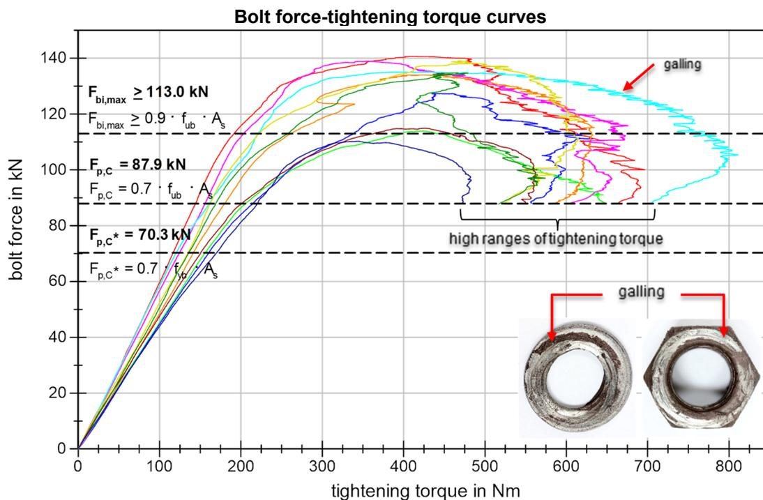
**Figure 84** BU\_M20\_88 Bolt force-tightening torque curves
