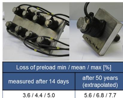
(d) loss preload measured/extrapolated after 14 days/ 50 years
