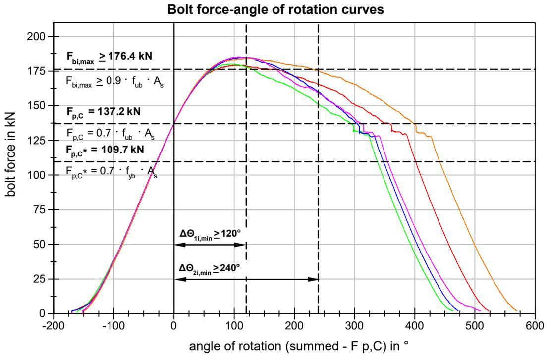
**Figure 56** BU\_M20\_88 (Gleitmo 1952V) Bolt force-angle of rotation curves
