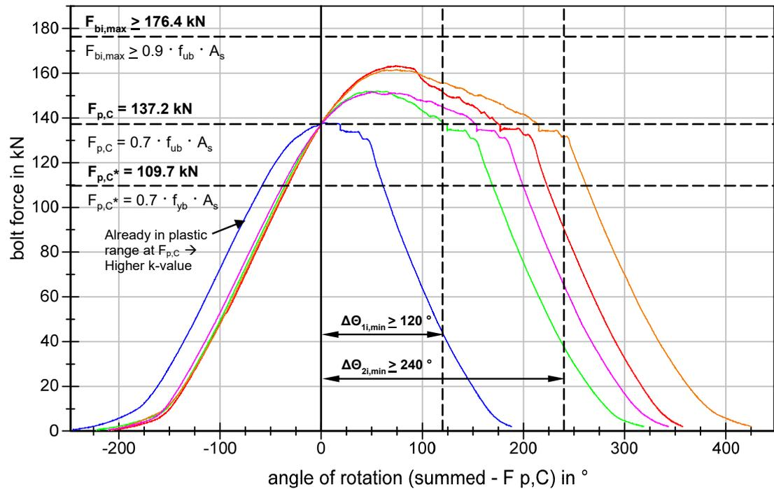
**Figure 38** BU\_M20\_88 (2013) Bolt force-angle of rotation curves
