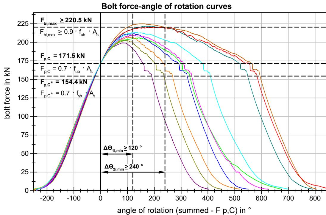
Figure 80 BU\_M20\_DX Bolt force-angle of rotation curves
