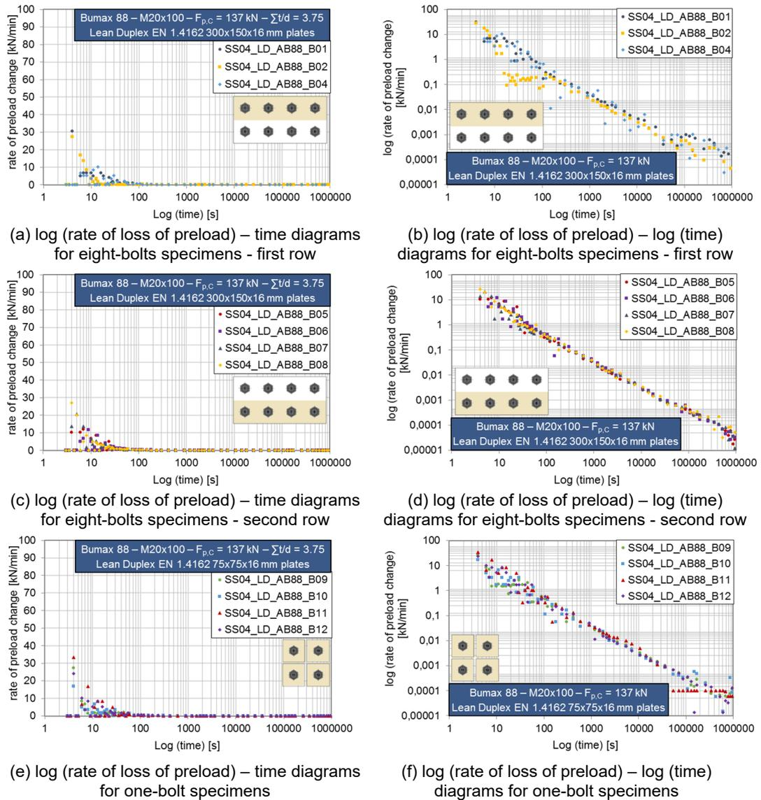
**Figure 183** Rate of loss of preload for SS04 test series (M20 bolting assemblies, preload level:  $F_{p,c}$  172 kN,  $\Sigma t/d = 3.75$ )
