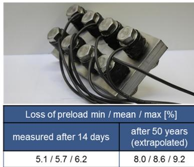
(c) loss preload measured/extrapolated after 14 days/ 50 years
