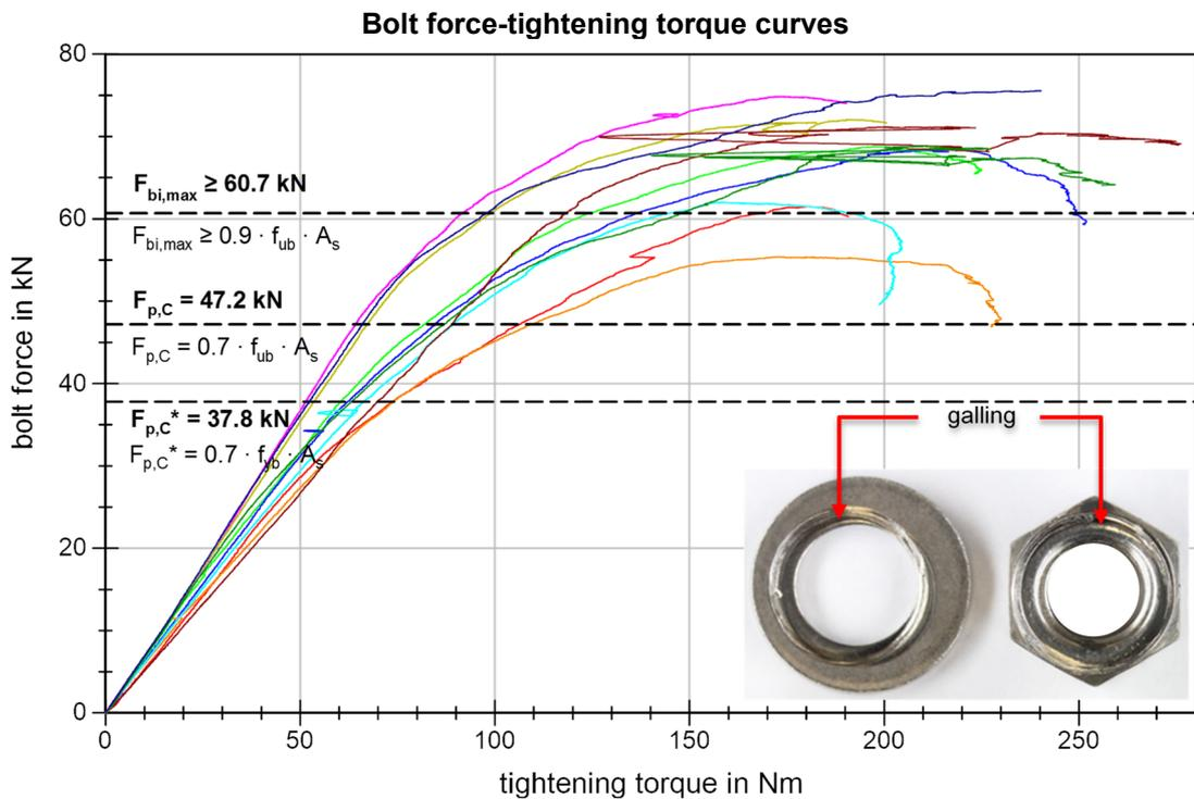
Figure 18 BU\_M12\_88 Bolt force-tightening torque curves
