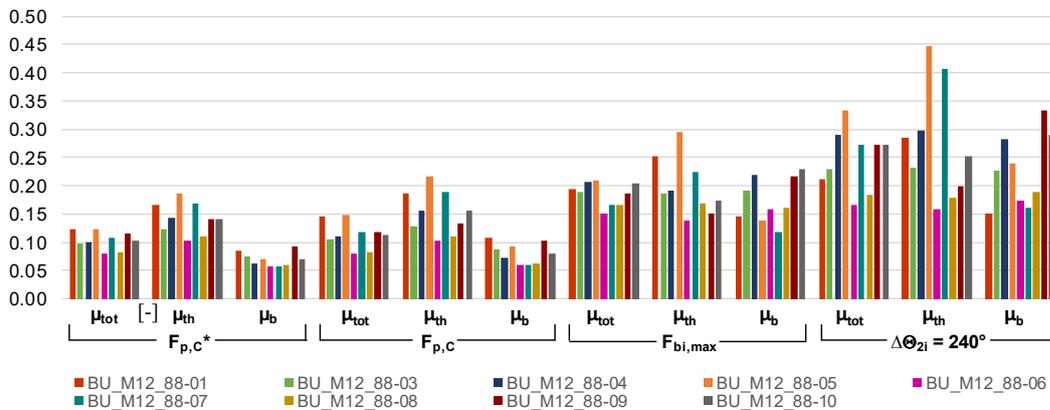
Figure 104 BU\_M12\_88 distribution of friction at selected bolt force levels
