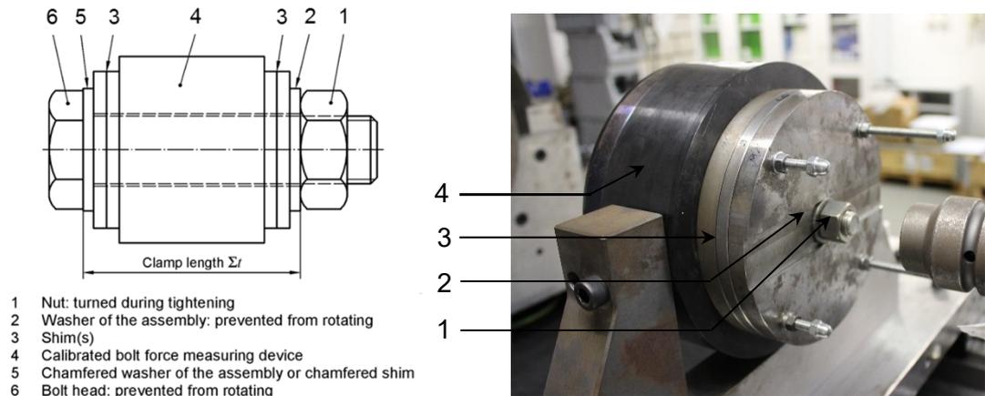
**Figure 12** Test setup for tightening tests at IML-UDE (exemplarily)
