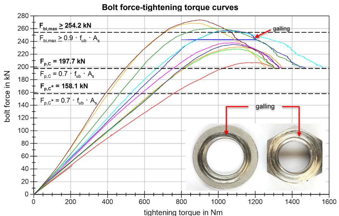
**Figure 54** BU\_M20\_88 (2015) Bolt force-tightening torque curves
