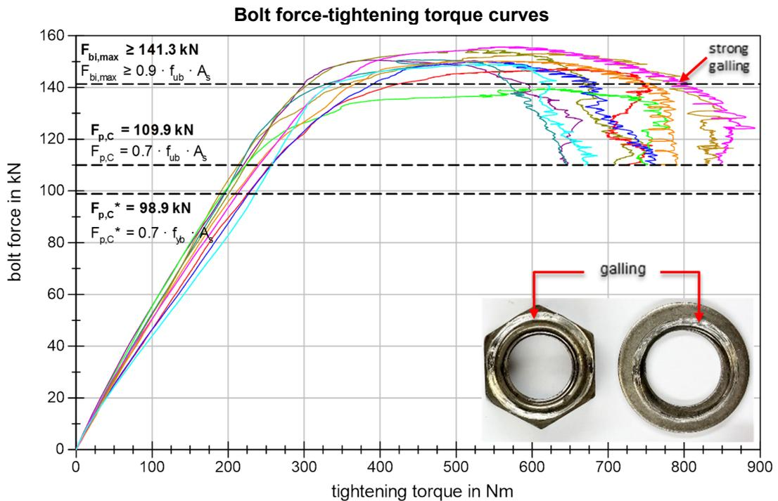
**Figure 93** BU\_M16\_LDX Bolt force-tightening torque curves
