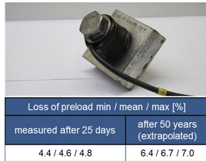
(b) loss preload measured/extrapolated after 20 days/ 50 years
