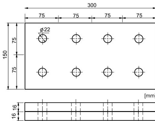
(c) Test specimen with eight M20 bolts
