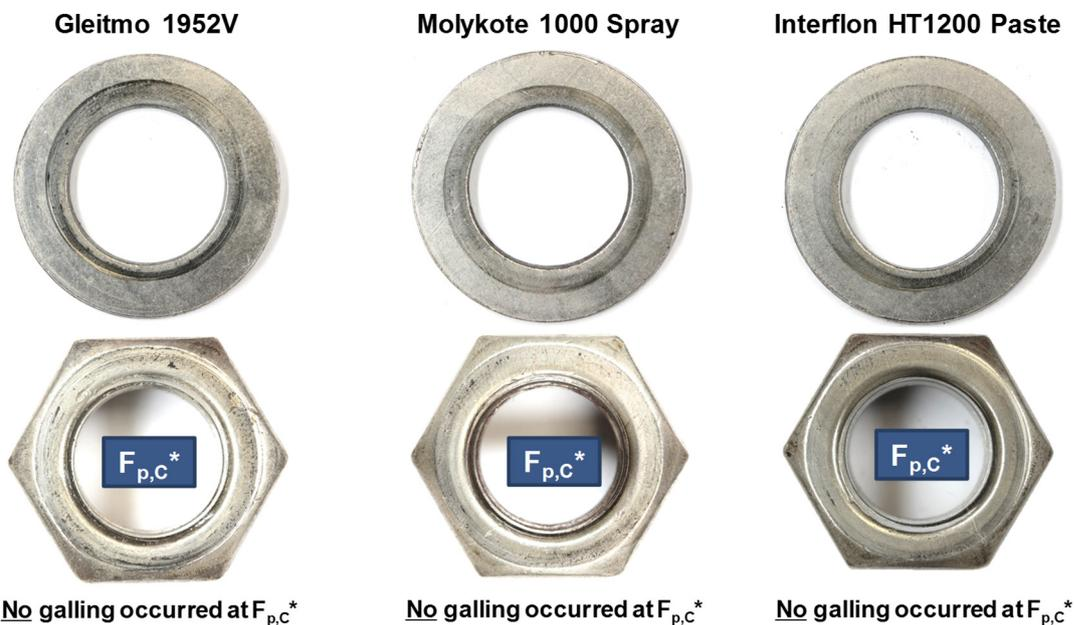
**Figure 115** Inspection of galling of austenitic M20 HV200 washers and M20 Bumax 88 austenitic nuts in property class 8.8 after tightening at specified preload level  $F_{p,C}^* = 0.7 f_{yb} A_s$
