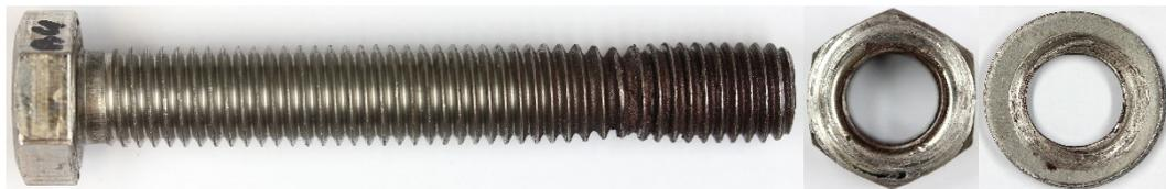
**Figure 70** BU\_M12\_SDX test specimen after tightening
