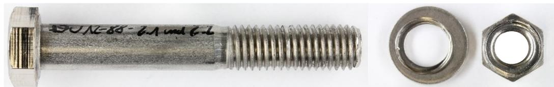
**Figure 16** BU\_M12\_88 test specimen after tightening
