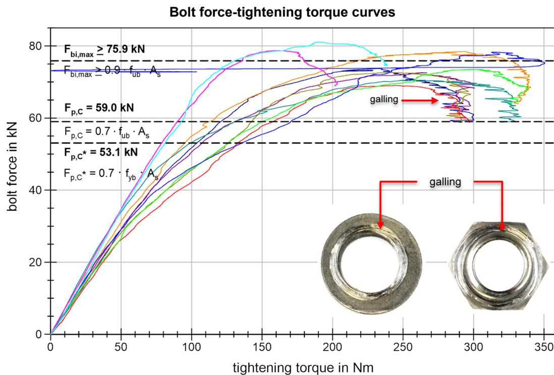
Figure 21 BU\_M12\_109 Bolt force-tightening torque curves
