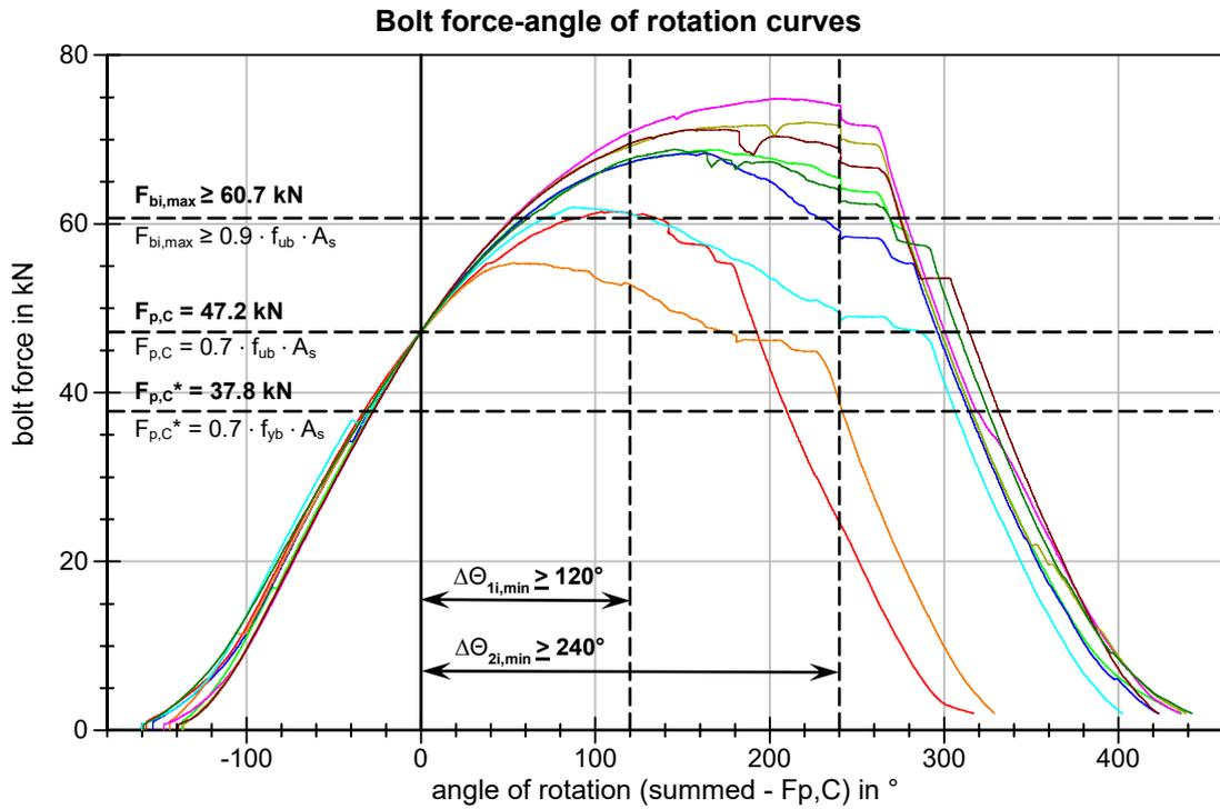
Figure 17 BU\_M12\_88 Bolt force-angle of rotation curves
