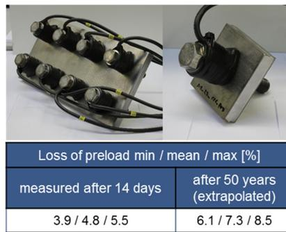
(d) loss preload measured/extrapolated after 14 days/ 50 years
