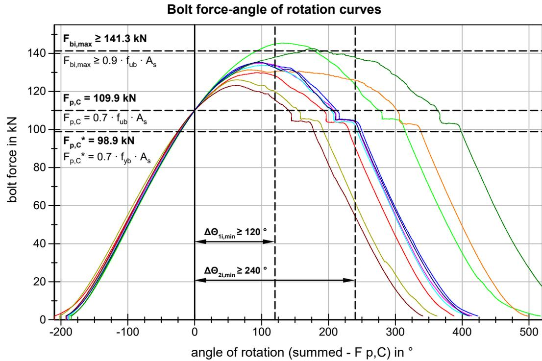
**Figure 35** BU\_M16\_DX Bolt force-angle of rotation curves
