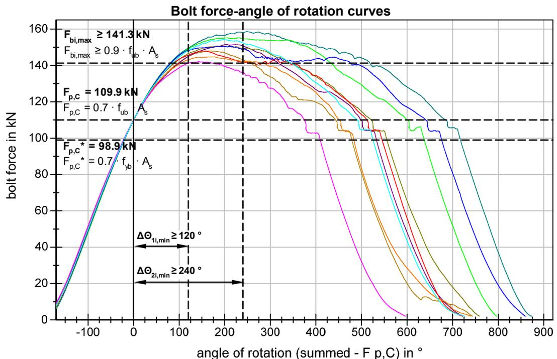
**Figure 95** BU\_M16\_DX Bolt force-angle of rotation curves
