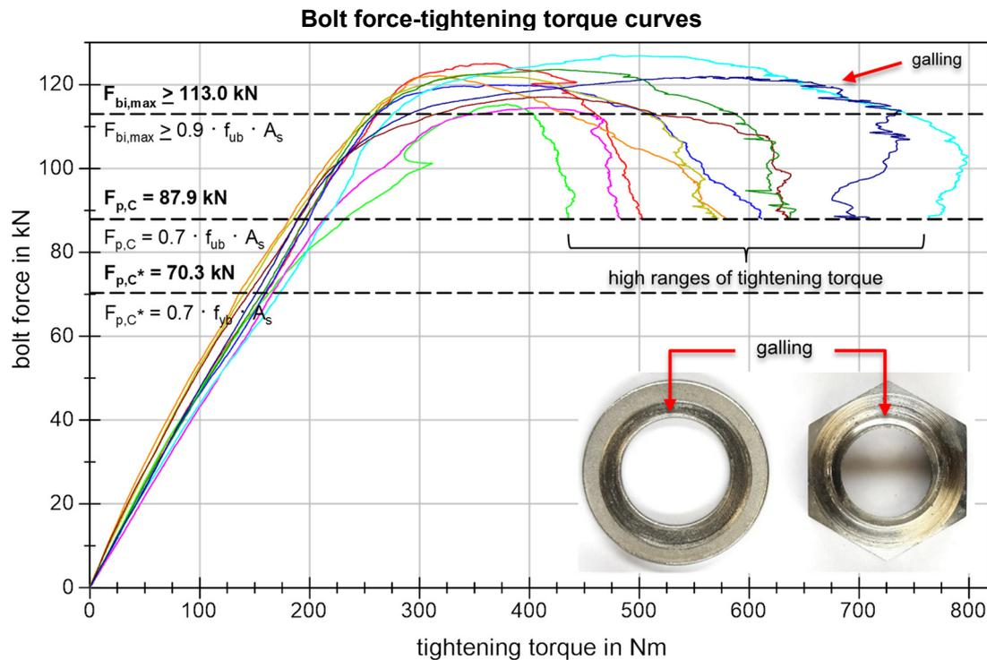
**Figure 27** BU\_M16\_88 Bolt force-tightening torque curves
