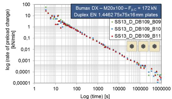
(b) log (rate of loss of preload) – log (time) diagrams for one-bolt specimens
