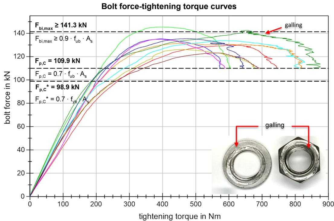
**Figure 36** BU\_M16\_DX Bolt force-tightening torque curves
