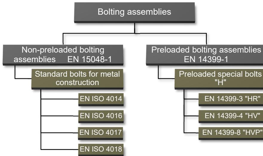
**Figure 1** Overview of bolting assemblies and harmonized standards used in the steel construction industry ([14][15])
