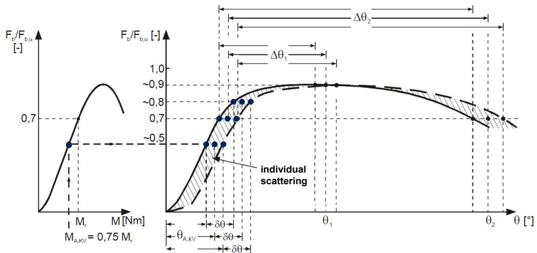
**Figure 10** Schematical overview of first and second tightening step of combined method acc. EN 1090-2:2011-10 [14] (© IML)
