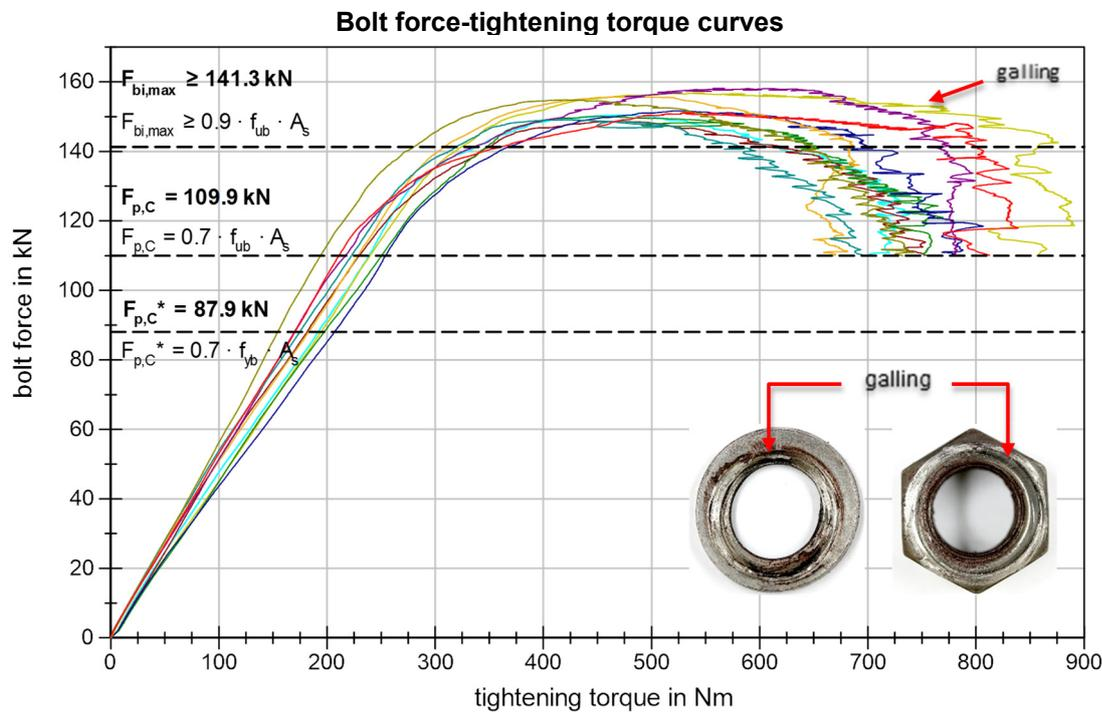
Figure 87 BU\_M16\_109 Bolt force-tightening torque curves
