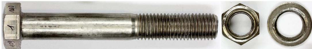
**Figure 43** BU\_M20\_109 test specimen after tightening
