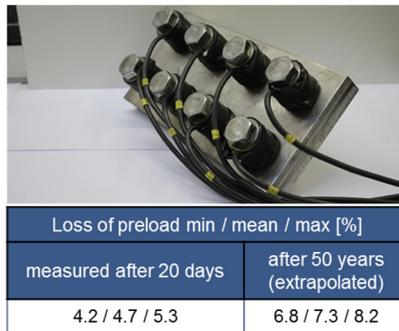
(c) loss preload measured/extrapolated after 20 days/ 50 years
