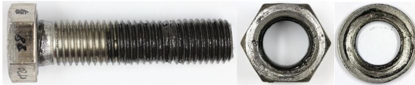
**Figure 64** BU\_M20\_DX test specimen after tightening
