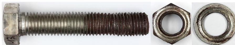
**Figure 73** BU\_M20\_109 test specimen after tightening
