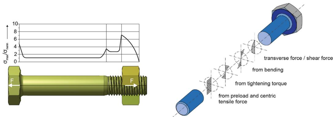
**Figure 5** Distribution and form factors  $\alpha_K$  of notches in a bolt (left) and stresses in bolt shank (right) (© IML for left and right Figure)
