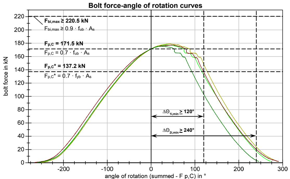
**Figure 44** BU\_M20\_109 bolt force-angle of rotation-curves (only specimens which achieved F<sub>p,c</sub>)
