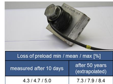
(b) loss preload measured/extrapolated after 10 days/ 50 years
