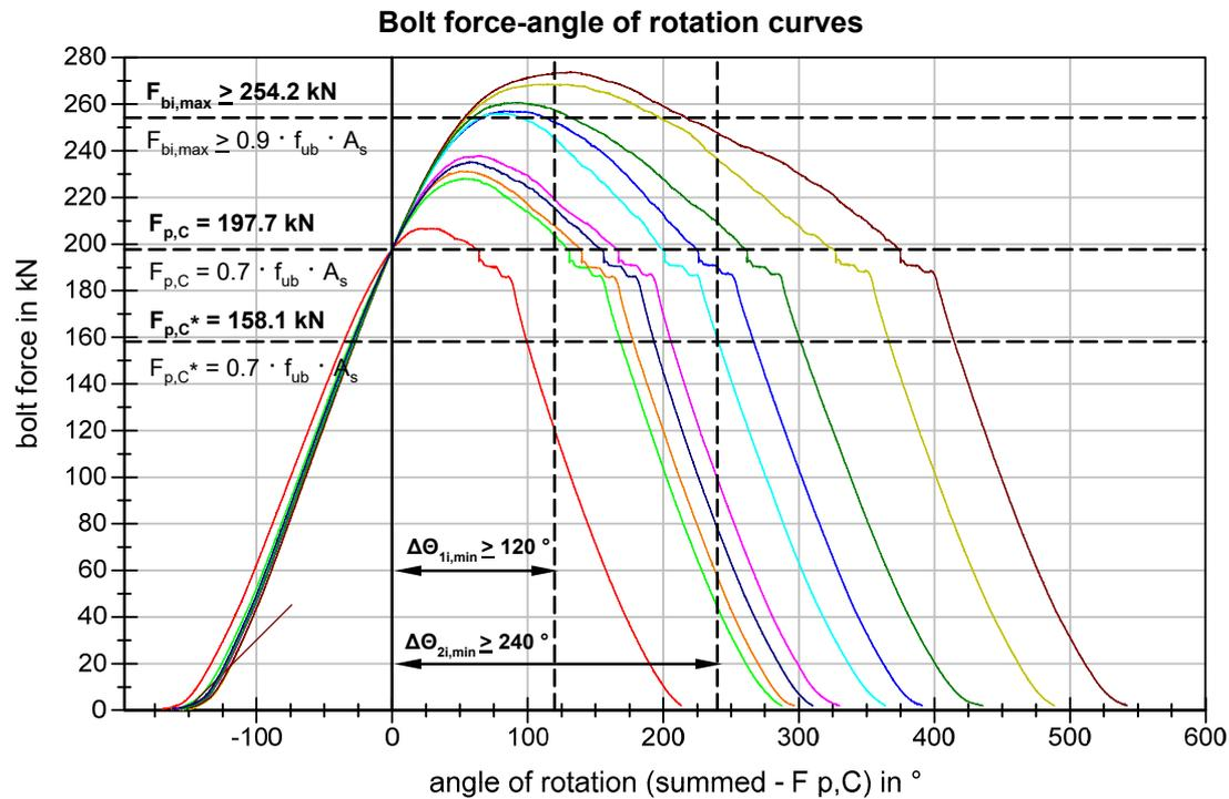
**Figure 53** BU\_M20\_88 (2015) Bolt force-angle of rotation curves
