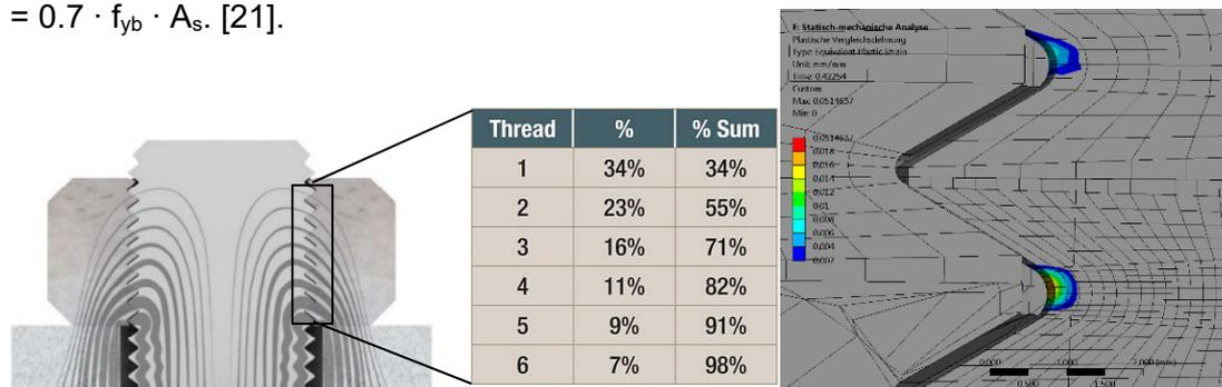
**Figure 6** Load distribution in the paired threads (left/middle) and plasticising at  $F_{p,C}^*$  (right)
