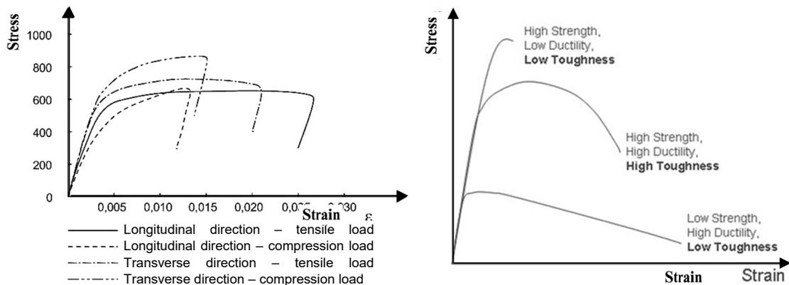
**Figure 9** Asymmetry and anisotropy of stainless steel (left) [23] and schematic overview of stress-strain behaviour depending on strength, ductility, and toughness (right) [© Ajax Bolt and Nut Co.]
