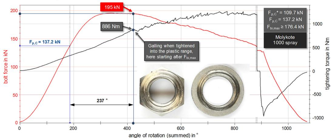
**Figure 110** BU\_M20\_88-07 – Example of minor galling in the tightening curves starting at maximum load
