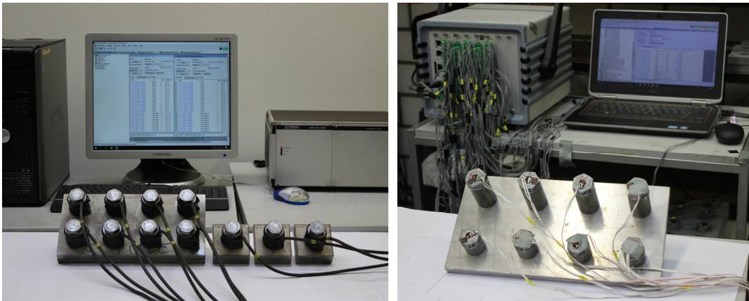
(a) performing relaxation test with load cells
