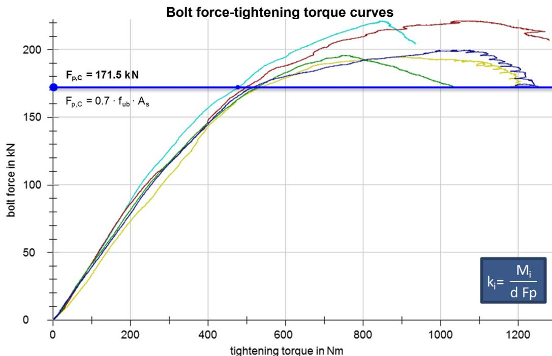
**Figure 102** BU\_M20\_LDX Bolt force-tightening torque curves – Interflon HT1200 paste
