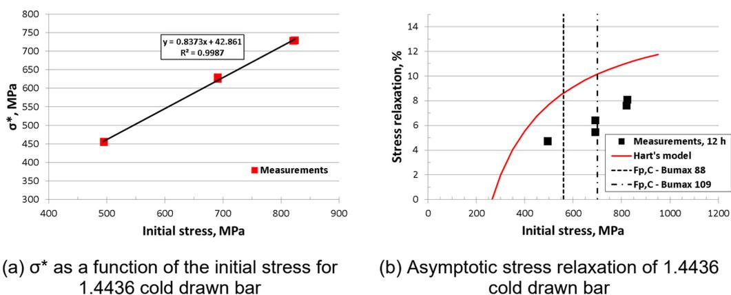
**Figure 136** Stress relaxation results fitted to the Hart's model for 1.4436 cold drawn bar material, see [1]/[29] and [29]
