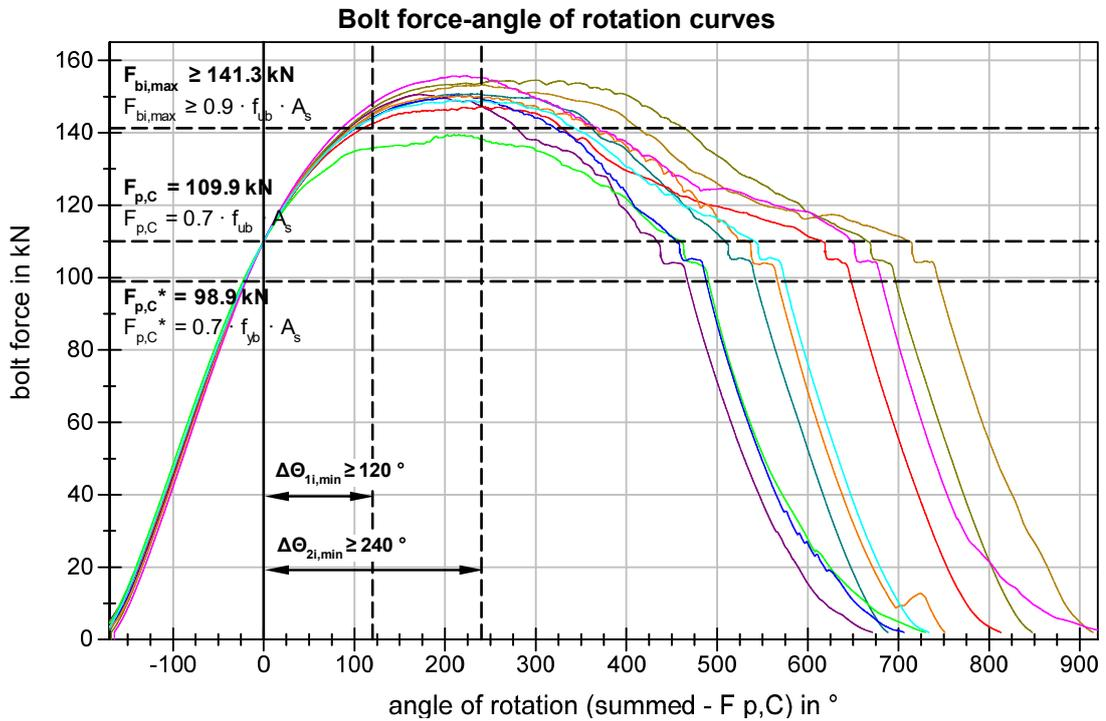
**Figure 92** BU\_M16\_LDX Bolt force-angle of rotation curves
