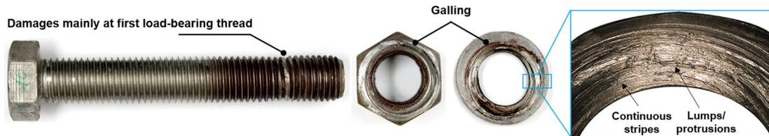
**Figure 103** Galling of the nut bearing surface when tightened into plastic range: bolt (left), nut and washer (middle), and detailed view of washer (right)
