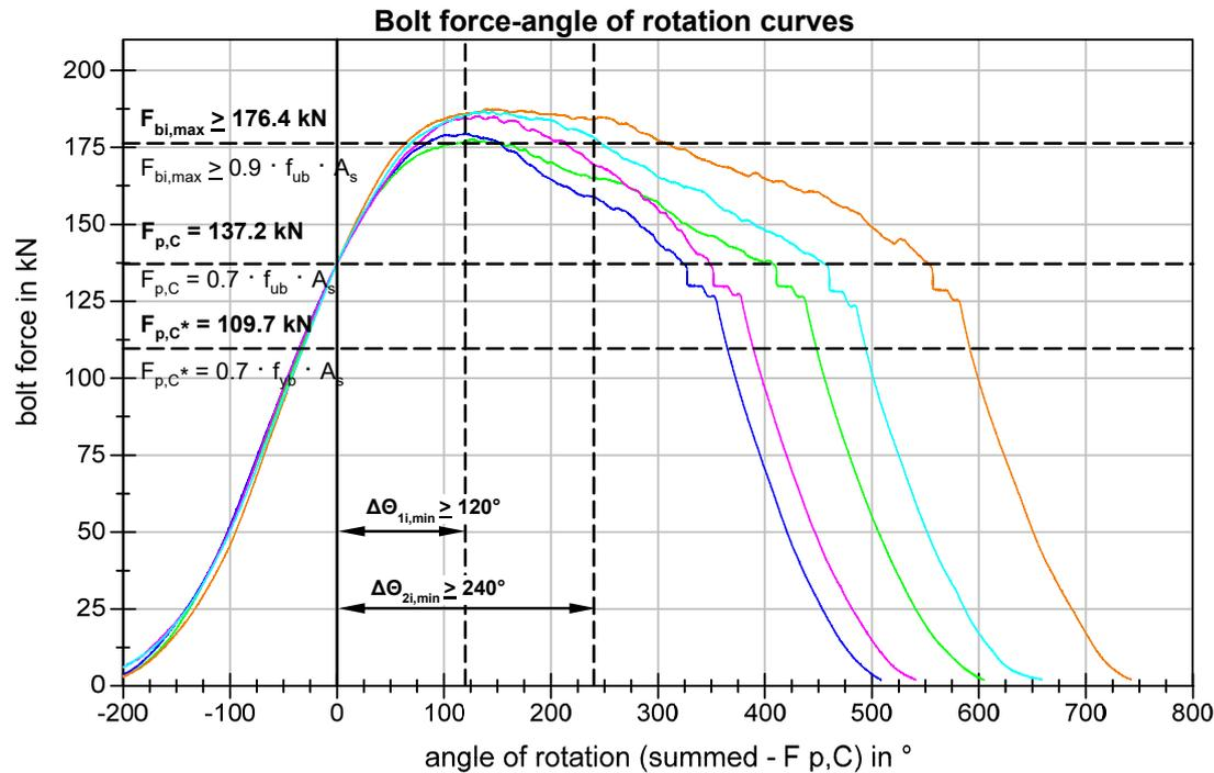
**Figure 65** BU\_M20\_88 (Molykote P-74 paste) Bolt force-angle of rotation curves
