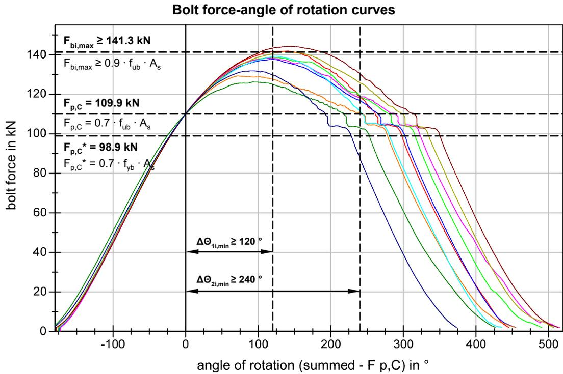
**Figure 32** BU\_M16\_LDX Bolt force-angle of rotation curves
