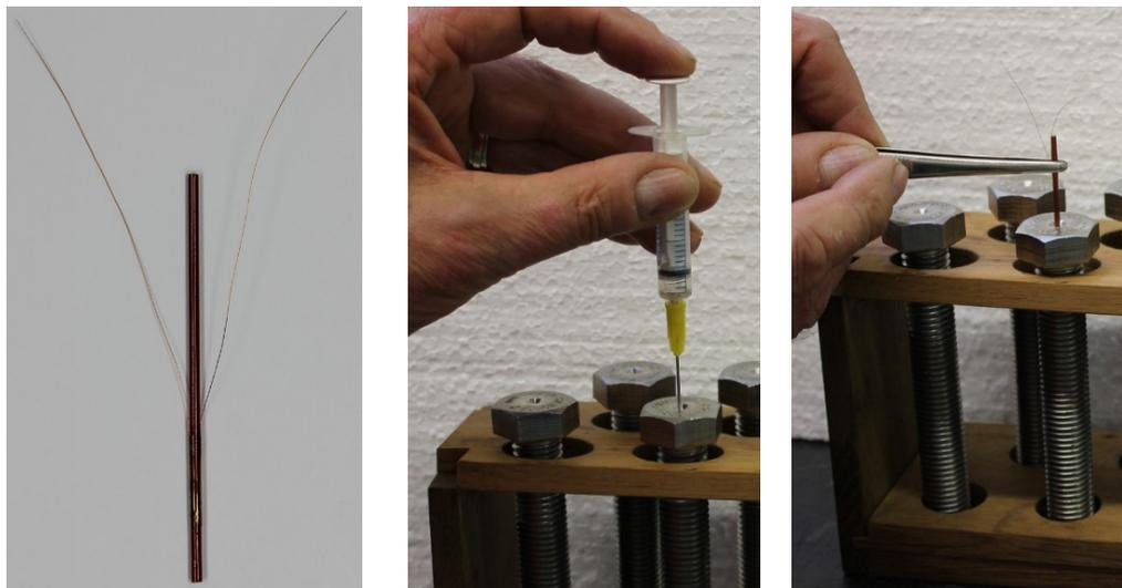
**Figure 119** Exemplary production phases of instrumented stainless steel bolts
