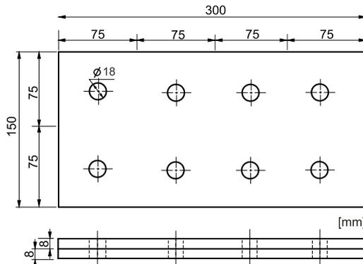
(a) Test specimen with eight M16 bolts
