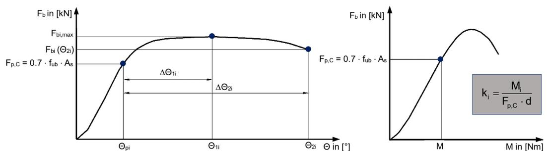
**Figure 14** Schematic bolt force-angle of rotation curve (left) and bolt force-tightening torque curve (right) according to EN 14399-2
