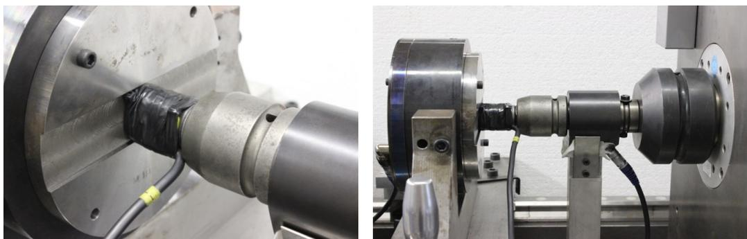
**Figure 123** Testing of the bolts with SG and LC in the tightening testing machine of the Institute for Metal and Lightweight Structures of University of Duisburg-Essen
