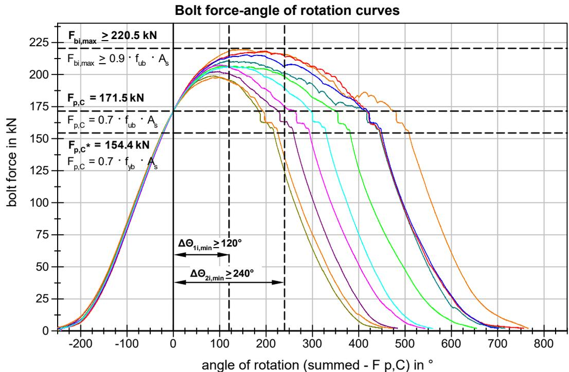
**Figure 77** BU\_M20\_LDX Bolt force-angle of rotation curves
