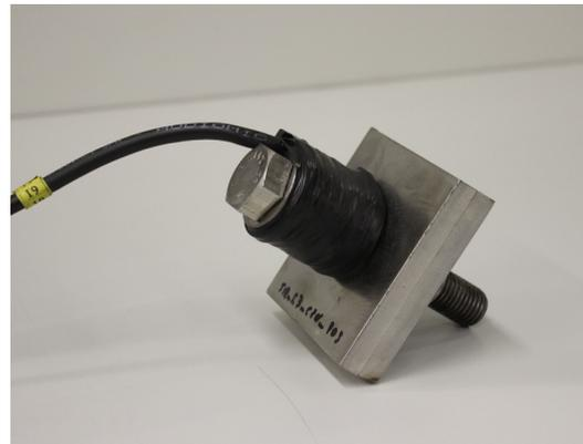
(f) One-bolt-specimen (75 mm × 75 mm plates)
