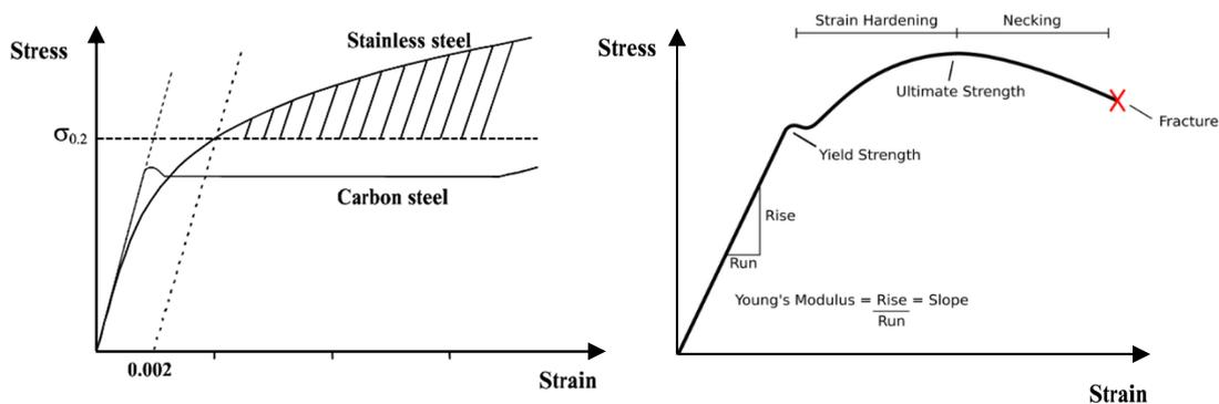
**Figure 8** Comparison of stress-strain curves for carbon steel and stainless steel (left) following [24] and characteristic values of stress-strain curves (right)
