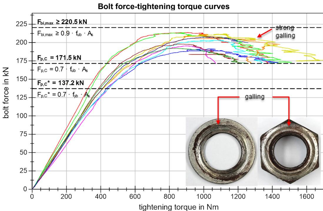
Figure 75 BU\_M20\_109 Bolt force-tightening torque curves
