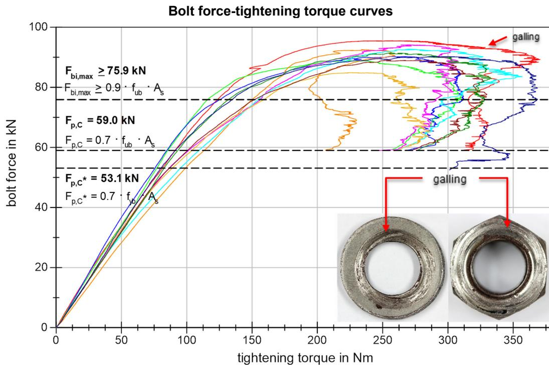
Figure 72 BU\_M12\_SDX Bolt force-tightening torque curves
