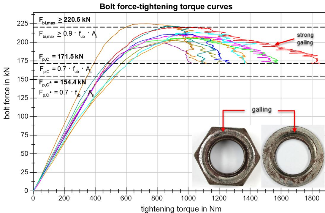
Figure 81 BU\_M20\_DX Bolt force-tightening torque curves
