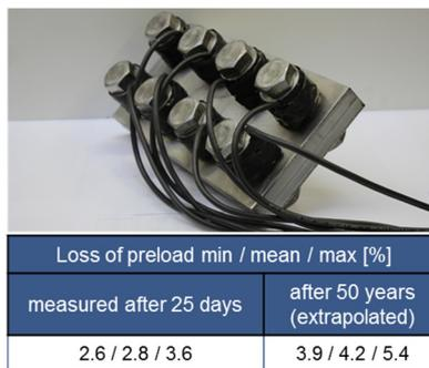
(c) loss preload measured/extrapolated after 25 days/ 50 years
