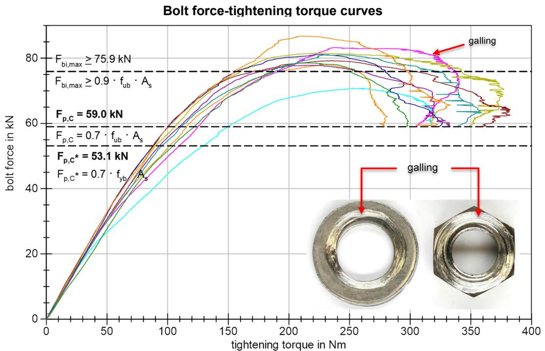
**Figure 24** BU\_M12\_SDX Bolt force-tightening torque curves
