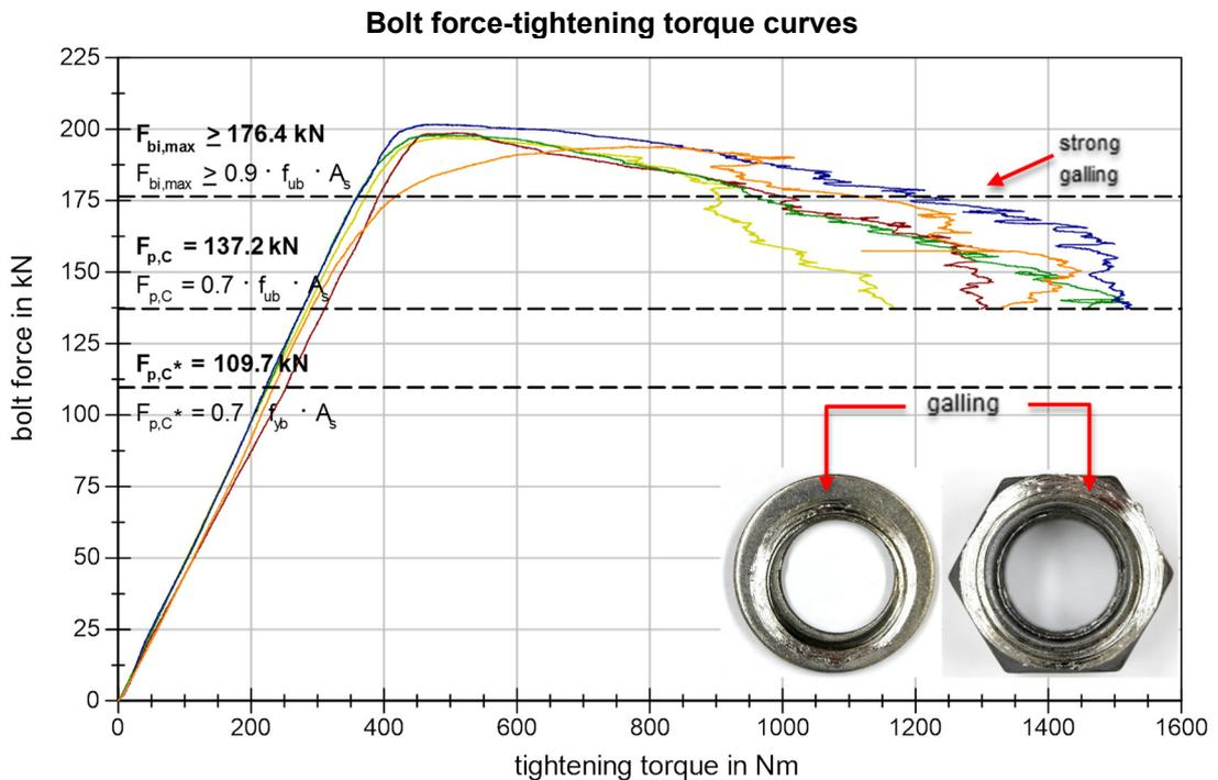
**Figure 69** BU\_M20\_88 (Molykote D-321R spray) bolt force-tightening torque curves
