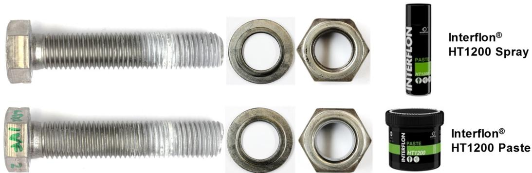
**Figure 114** Bumax – M20x100 bolting assemblies after tightening with Interflon HT1200 spray (above) and Interflon HT1200 paste (below)
