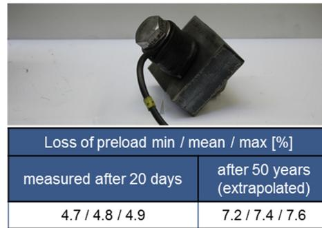
(b) loss preload measured/extrapolated after 20 days/ 50 years
