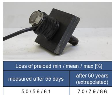
(b) loss preload measured/extrapolated after 55 days/ 50 years
