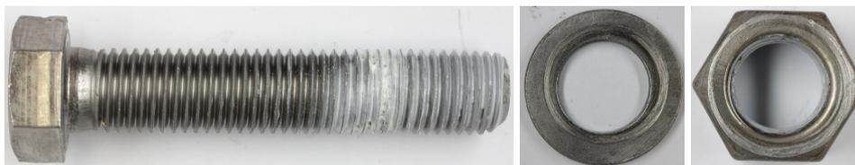
**Figure 100** BU\_M20\_LDX test specimen after tightening – Interflon HT1200 paste
