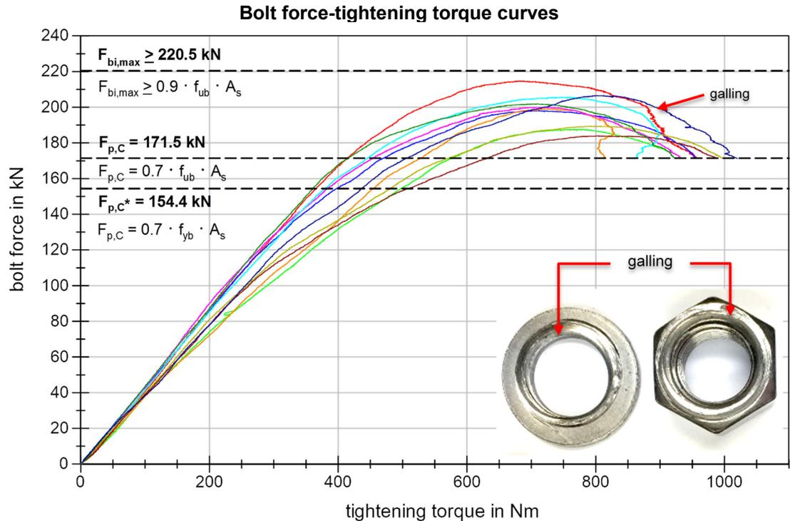
**Figure 48** BU\_M20\_LDX Bolt force-tightening torque curves
