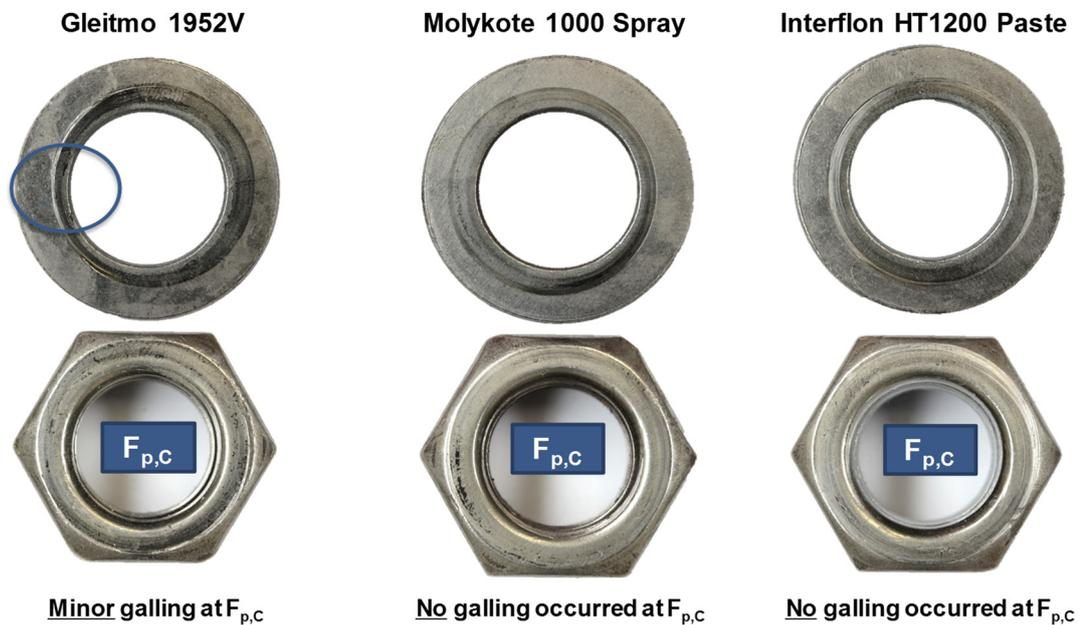
**Figure 116** Inspection of galling of austenitic M20 HV200 washers and M20 Bumax 88 austenitic nuts in property class 8.8 after tightening at specified preload level  $F_{p,C} = 0.7 f_{ub} A_s$
