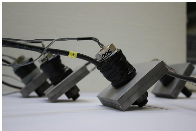
**Figure 125** Relaxation test samples (combination of strain gauge and load cell)
