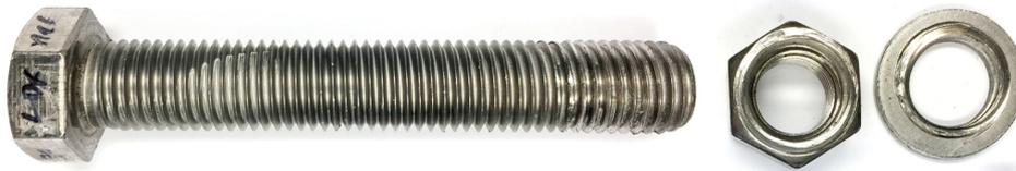
**Figure 31** BU\_M16\_LDX test specimen after tightening
