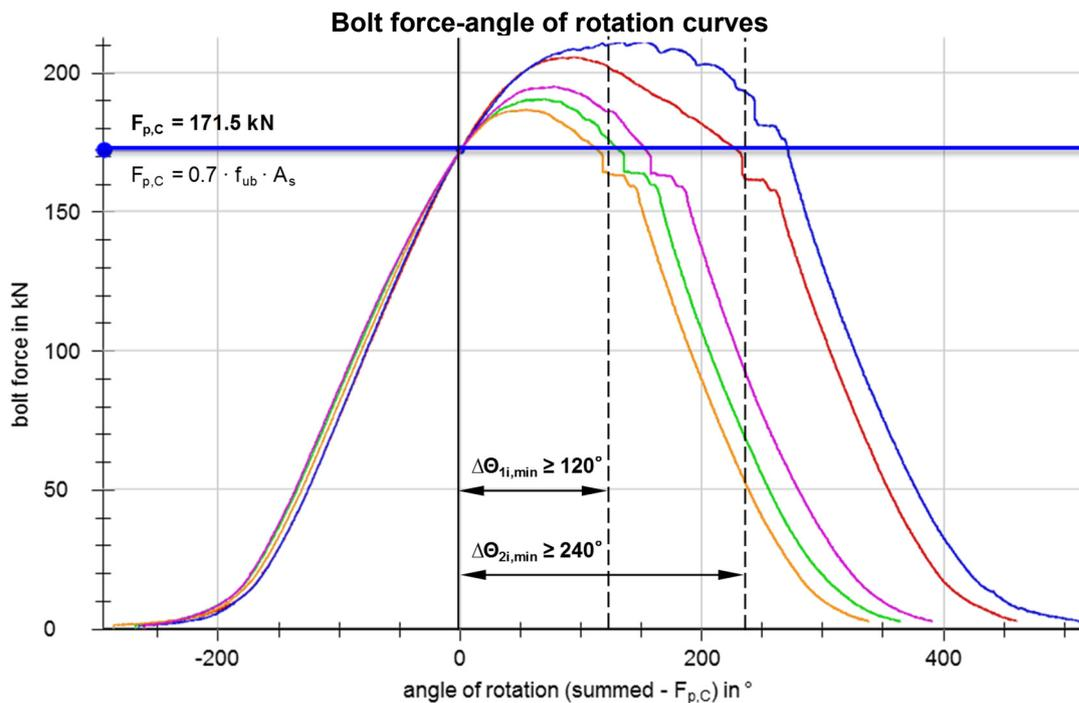
**Figure 98** BU\_M20\_LDX Bolt force-angle of rotation curves – Interflon HT1200 spray
