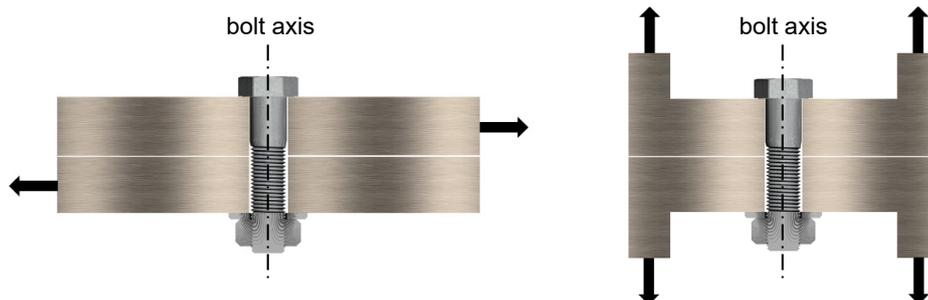
**Figure 2** Bolted shear connection (left) and tension connection (right)
