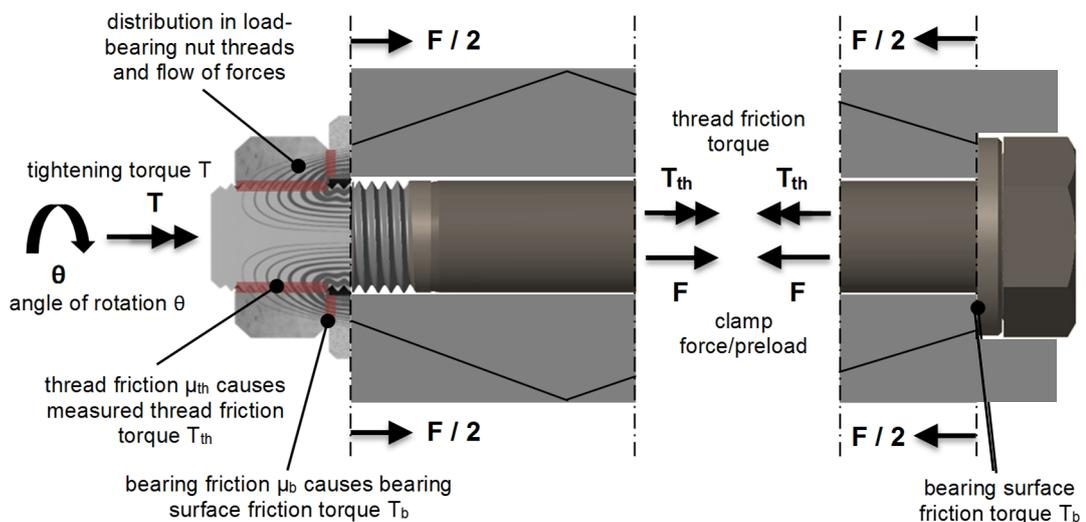
**Figure 4** Forces, torques and friction conditions in a bolted HV connection when tightened [19],[20]
