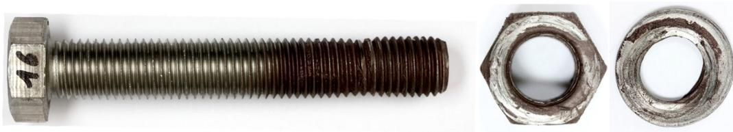
**Figure 82** BU\_M16\_88 test specimen after tightening
