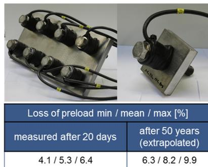
(d) loss preload measured/extrapolated after 20 days/ 50 years
