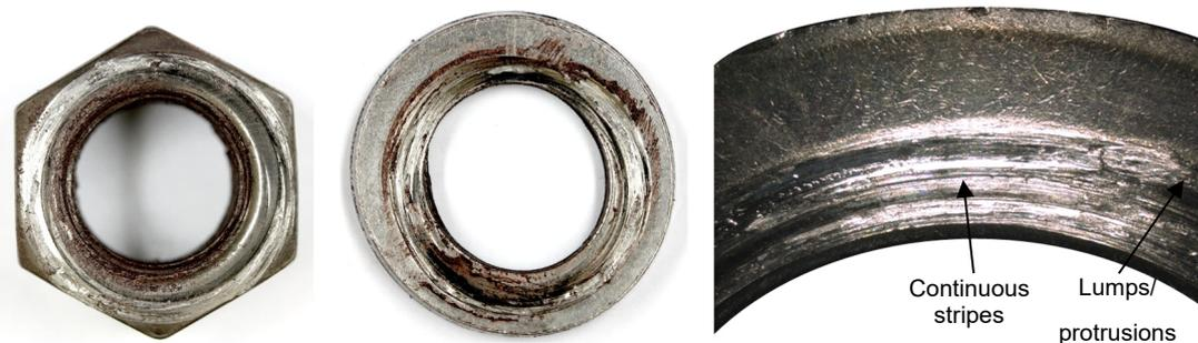
**Figure 109** Galling of the nut bearing surface when tightened into plastic range: nut (left), washer (middle) and detailed view of washer (right)
