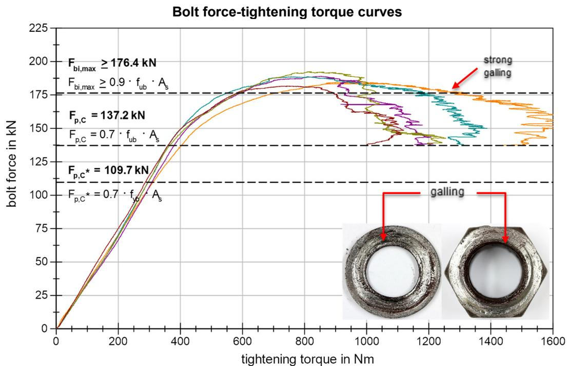
**Figure 63** BU\_M20\_88 (Molykote 1000 paste) Bolt force-tightening torque curves
