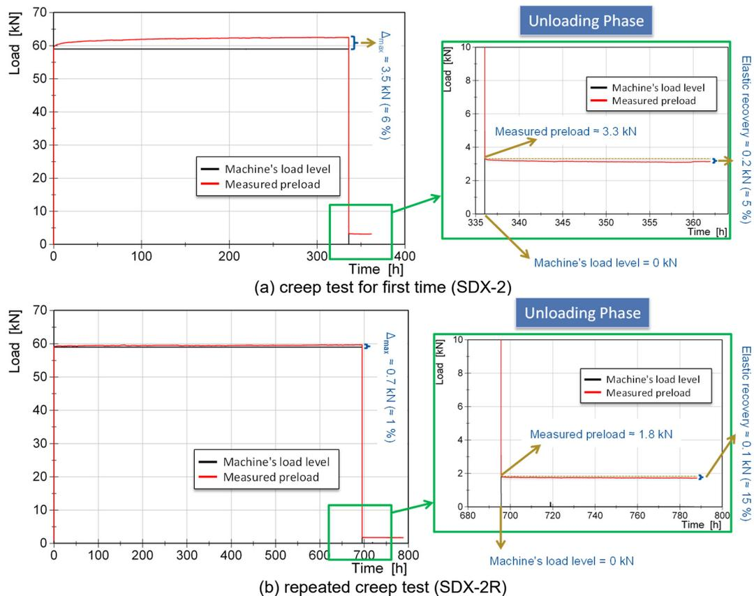
**Figure 121** Creep test M12 super duplex bolt
