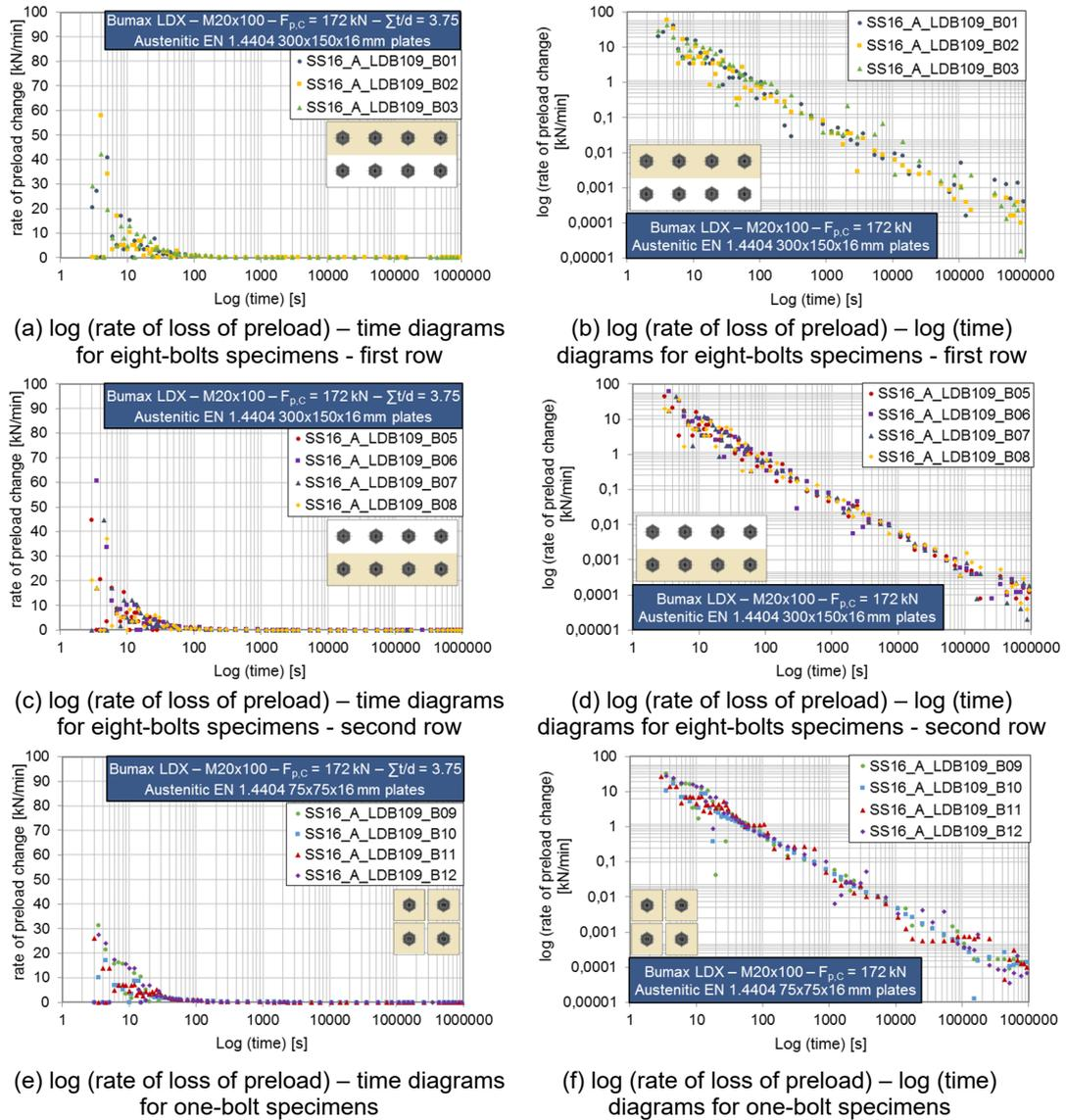
**Figure 134** Exemplary rate of loss of preload for SS16 test series (M20 bolting assemblies, preload level:  $F_{p,C}$  172 kN,  $\Sigma t/d = 3.75$ )
