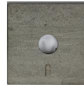
(b) One-bolt austenitic specimens in 1D surface condition
