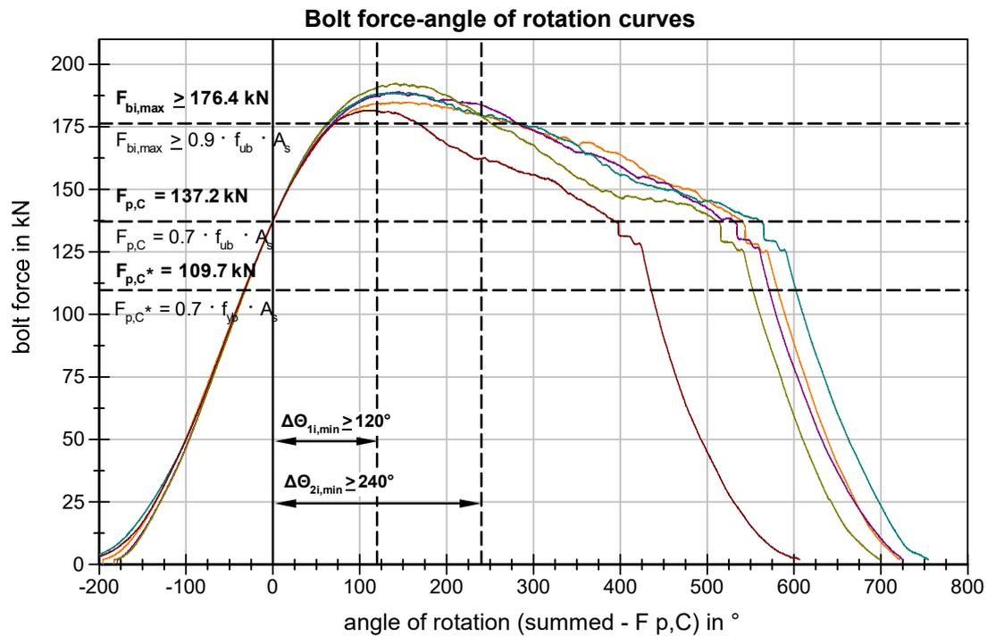
**Figure 62** BU\_M20\_88 (Molykote 1000 paste) Bolt force-angle of rotation curves
