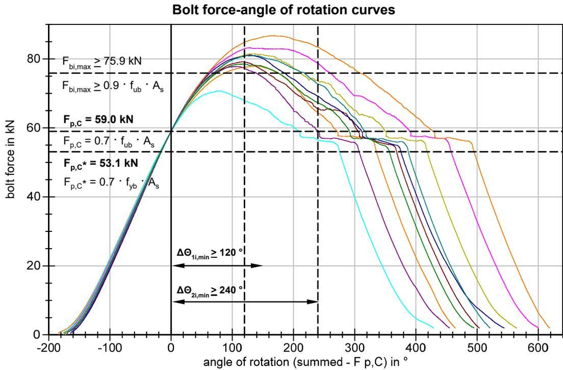
**Figure 23** BU\_M12\_SDX Bolt force-angle of rotation curves
