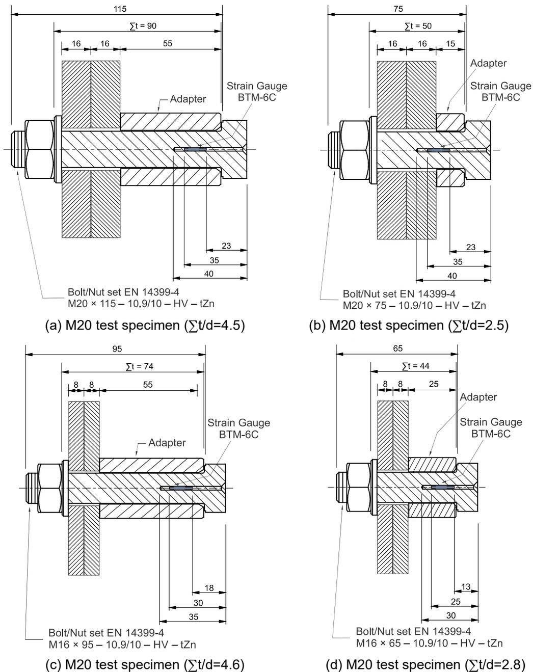
**Figure 129** Clamping length of the carbon steel HV-bolting assemblies for the relaxation test tests in two different clamping lengths for each bolt dimension
