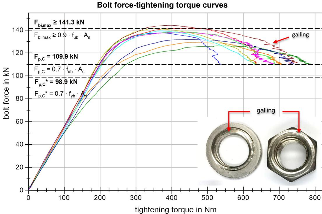
**Figure 33** BU\_M16\_LDX Bolt force-tightening torque curves
