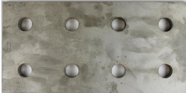
(a) Eight-bolts duplex specimens in 1D surface condition
