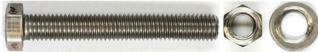
**Figure 22** BU\_M12\_SD\_X test specimen after tightening
