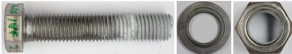
**Figure 97** BU\_M20\_LDX test specimen after tightening – Interflon HT1200 spray
