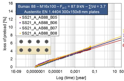
(b) preload losses-log (time) diagrams for eight-bolts specimens - second row
