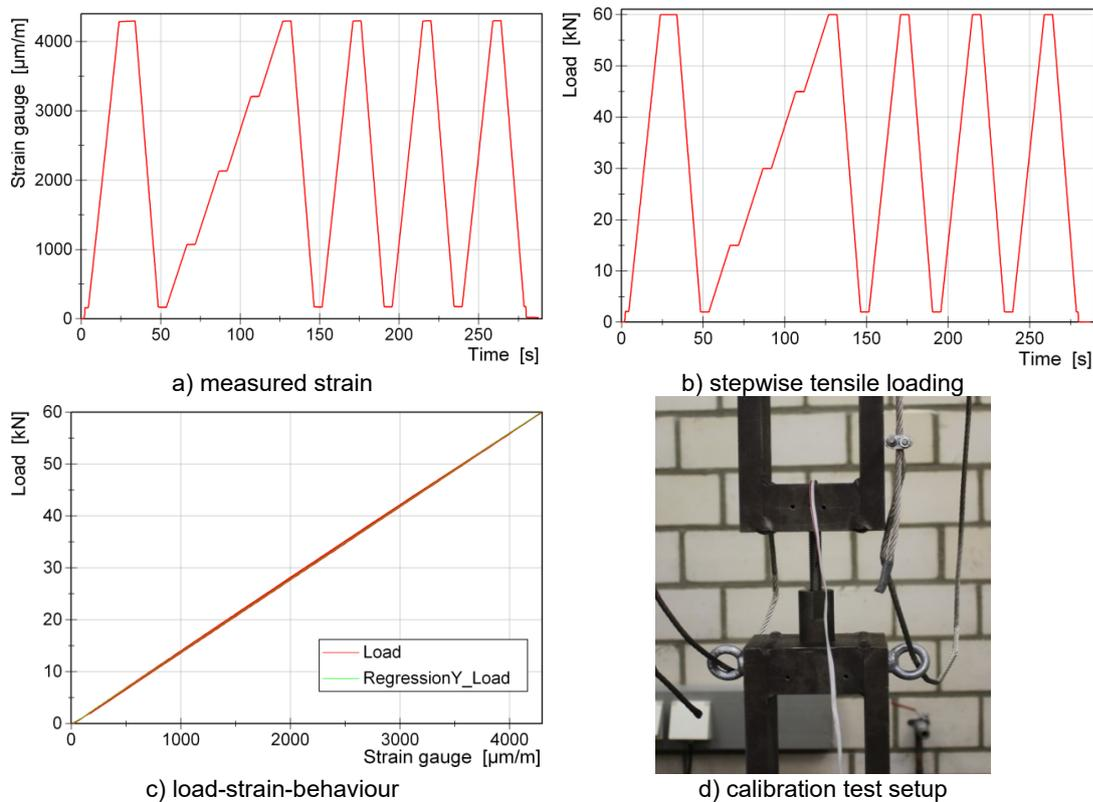
**Figure 120** Calibration of instrumented M12 super duplex bolt
