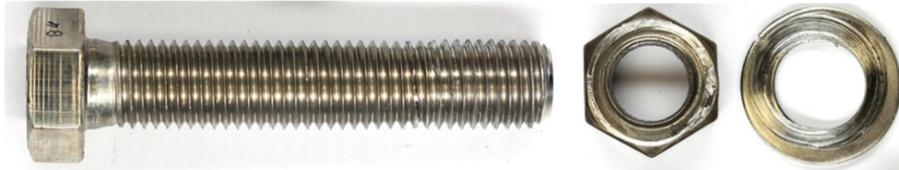
**Figure 37** BU\_M20\_88 (2013) test specimen after tightening
