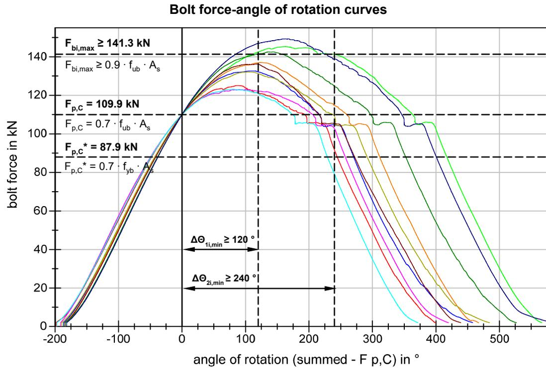
**Figure 29** BU\_M16\_109 Bolt force-angle of rotation curves
