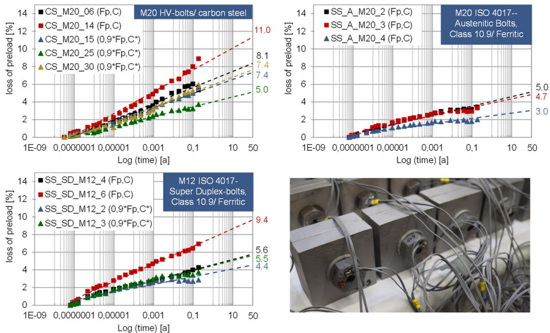
**Figure 124** Preload losses after 50 years in preload losses-log (time) diagrams exemplary for M20 HV-bolts in a clamping package made of carbon steel as well as austenitic M20-ISO 4017 bolts and super duplex M20 ISO 4017 bolts, each in clamping packages made of ferritic stainless steel; presentation of the test samples
