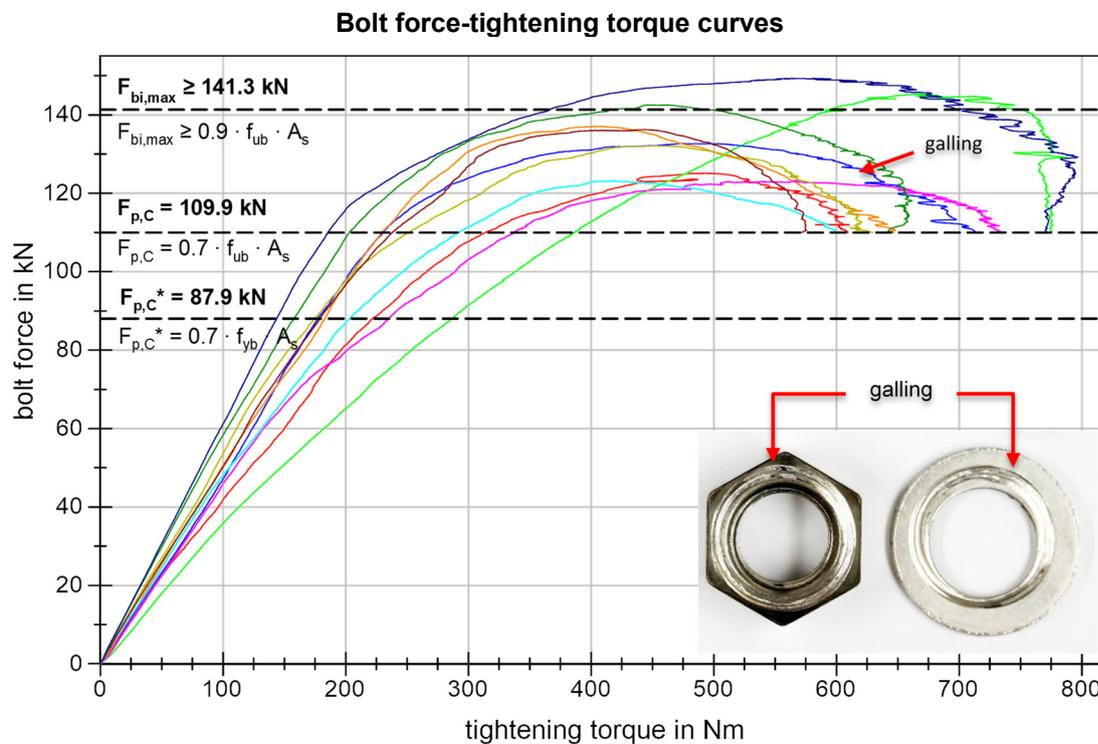
**Figure 30** BU\_M16\_109 Bolt force-tightening torque curves
