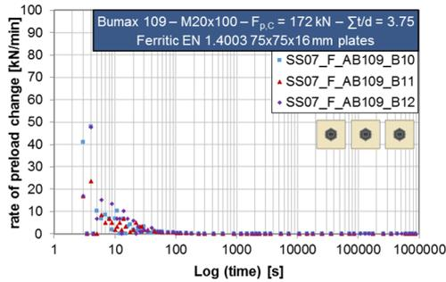
(a) log (rate of loss of preload) – time diagrams for one-bolt specimens
