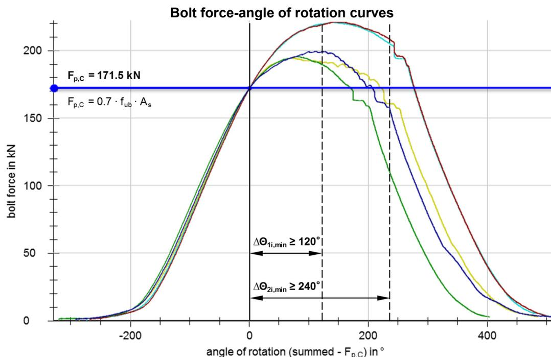
**Figure 101** BU\_M20\_LDX Bolt force-angle of rotation curves – Interflon HT1200 paste
