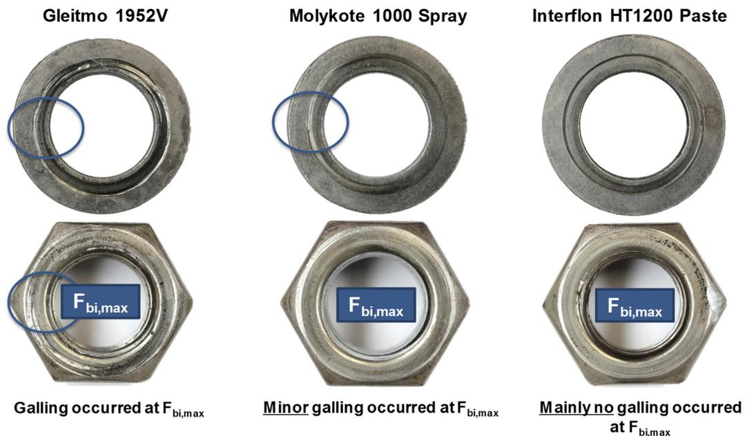
**Figure 117** Inspection of galling of austenitic M20 HV200 washers and M20 Bumax 88 austenitic nuts in property class 8.8 after tightening at specified preload level  $F_{bi,max} \geq 0.9 f_{ub} A_s$
