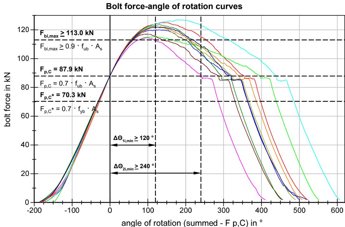
**Figure 26** BU\_M16\_88 Bolt force-angle of rotation curves
