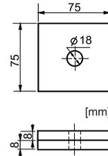
(b) Test specimen with one M16 bolt
