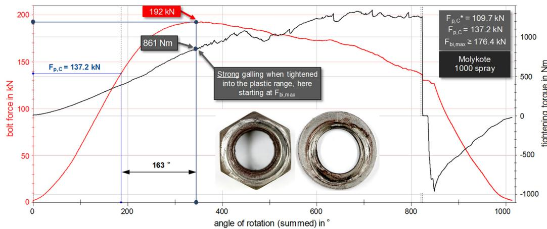
**Figure 111** BU\_M20\_88-09 – Example of major galling in the tightening curves starting at maximum load
