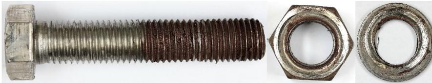
**Figure 76** BU\_M20\_LDX test specimen after tightening
