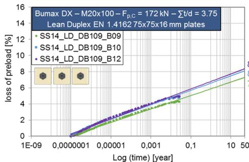
(a) preload losses-log (time) diagrams for one-bolt specimens
