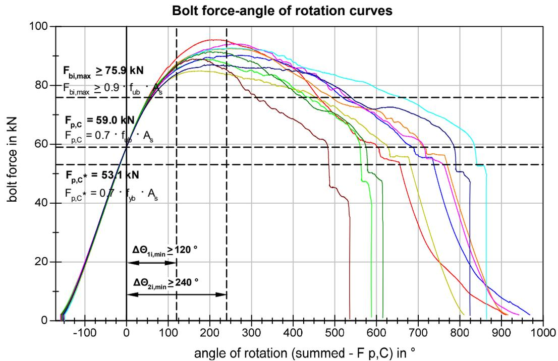
Figure 71 BU\_M12\_SDX Bolt force-angle of rotation curves
