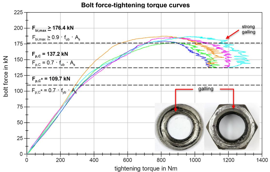
**Figure 66** BU\_M20\_88 (Molykote P-74 paste) Bolt force-tightening torque curves
