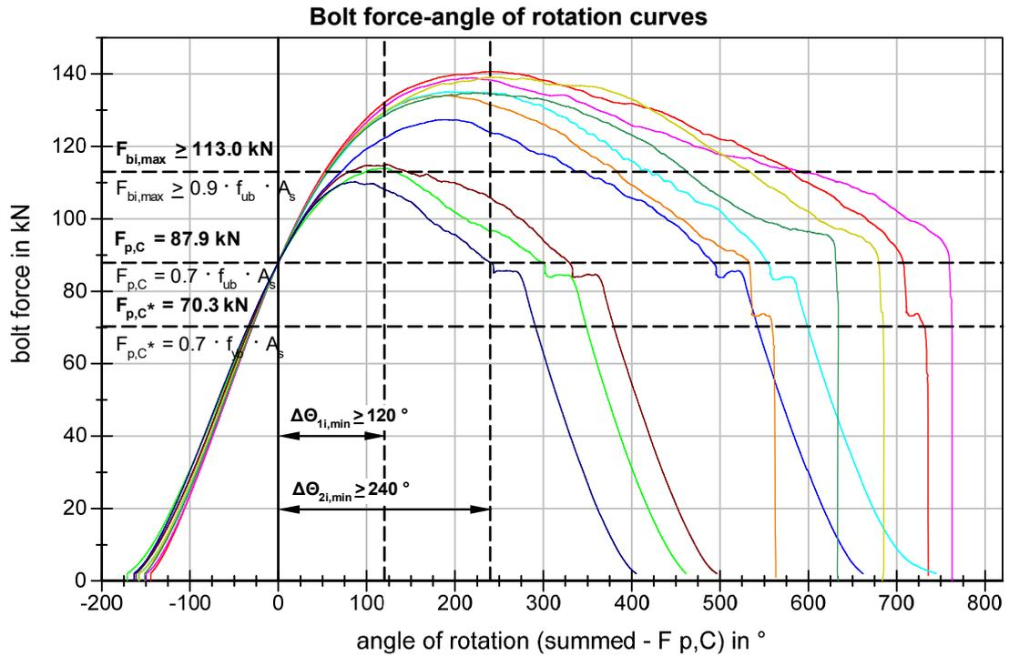
**Figure 83** BU\_M20\_88 Bolt force-angle of rotation curves
