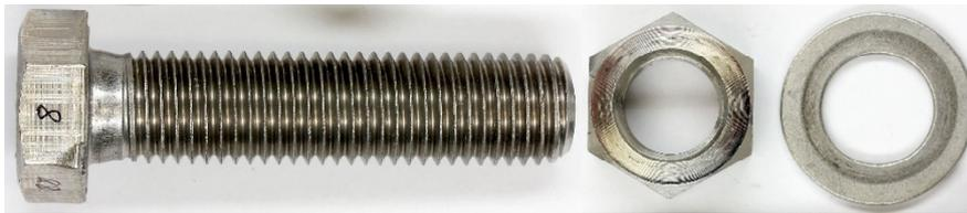
**Figure 52** BU\_M24\_88 test specimen after tightening
