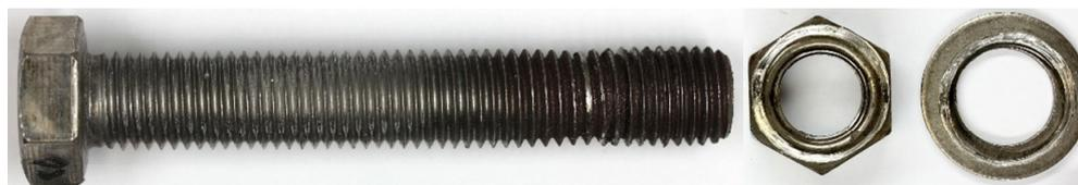
**Figure 91** BU\_M16\_LDX test specimen after tightening
