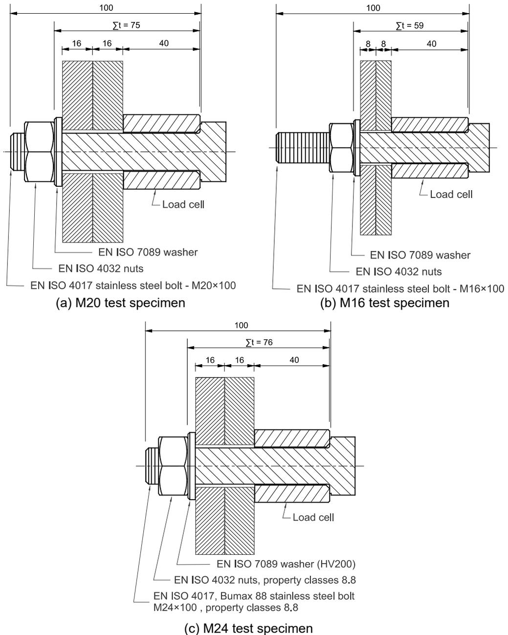
**Figure 128** Clamping length of the stainless steel bolting assemblies for the relaxation test tests
