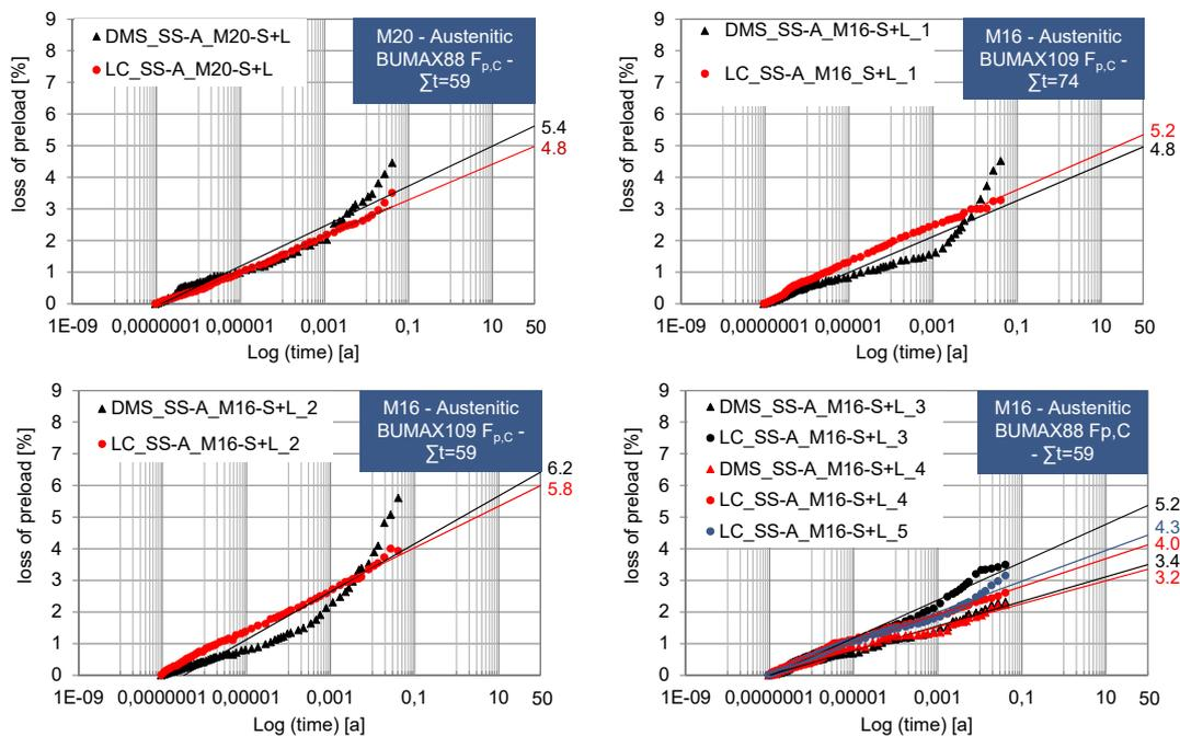
**Figure 126** Preload losses after 50 years in preload losses-log (time) diagrams for M20 and M16 Austenitic-bolts
