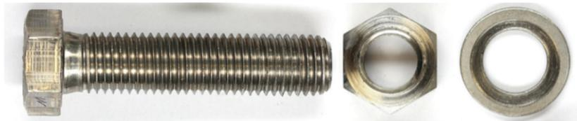
**Figure 25** BU\_M16\_88 test specimen after tightening
