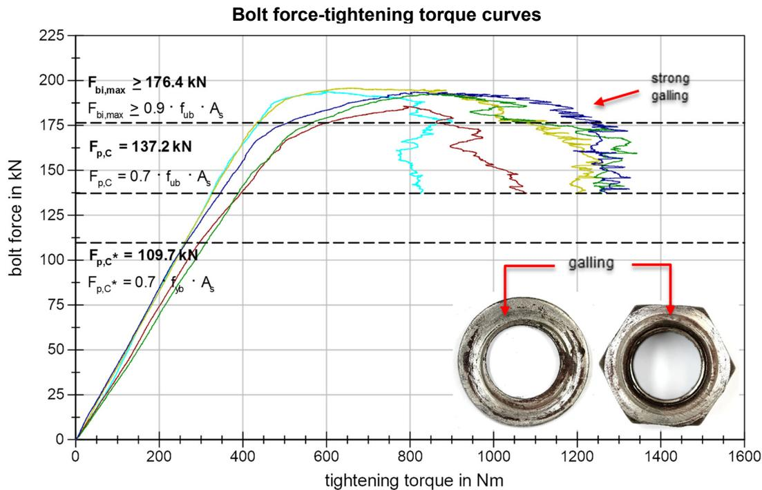
**Figure 60** BU\_M20\_88 (Molykote 1000 spray) Bolt force-tightening torque curves
