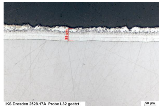
(h) sweep blasting 0.2-0.5 mm particle size - outer plate
