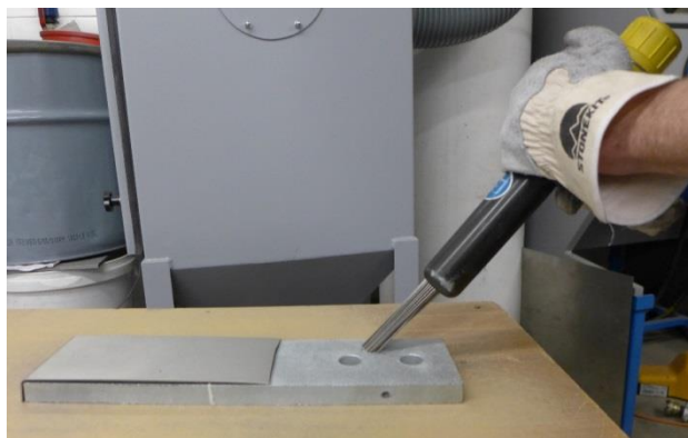
(a) needle gun at an angle of 45° to the zinc surface
