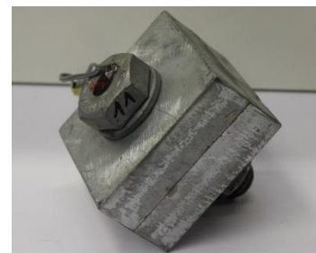
Figure 14 Test specimen geometry and test setup for the relaxation tests of the bolted connections
