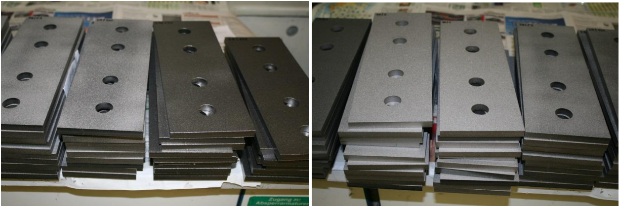
Figure 20 - Test pieces after blast-cleaning
