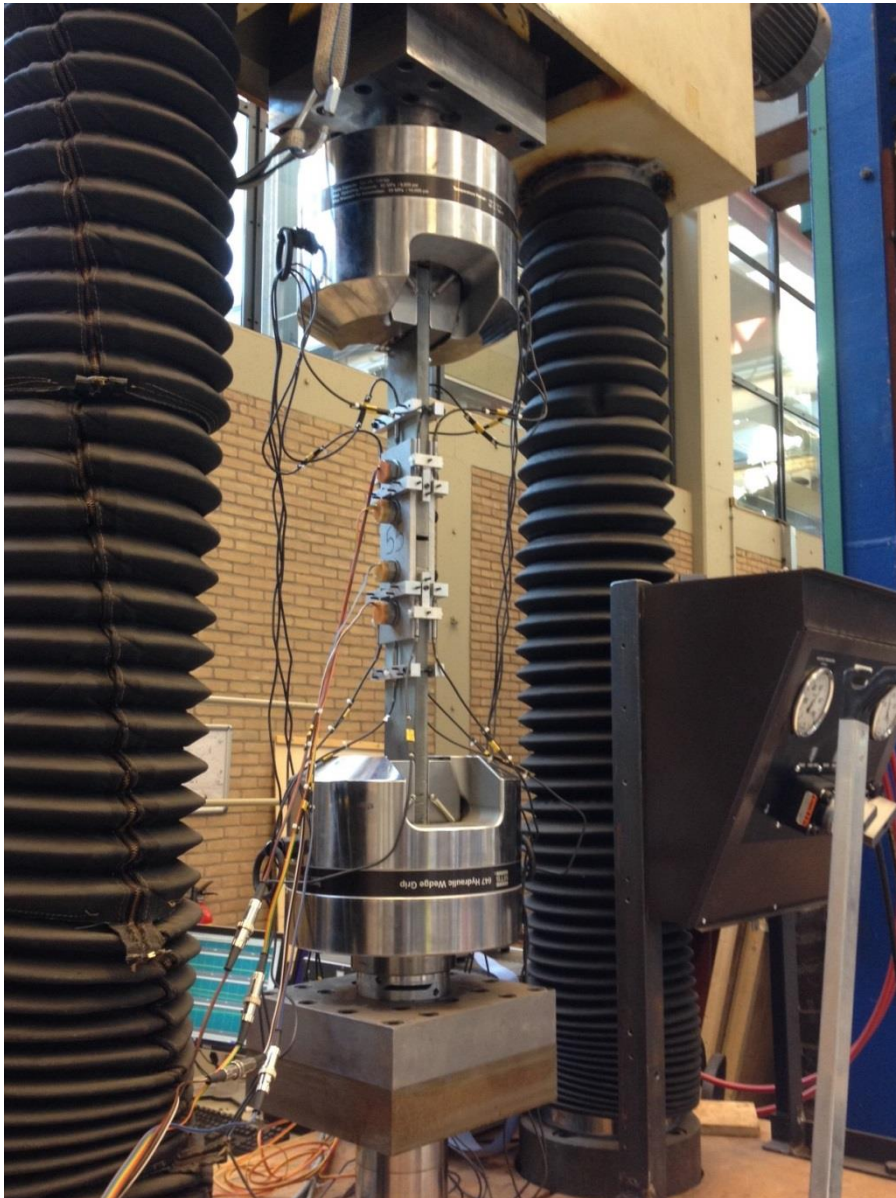
Figure 15 - Overview of test setup (600kN Schenck general purpose testing machine with MTS hydraulic clamping devices). Slip factor test specimen ready for testing.
