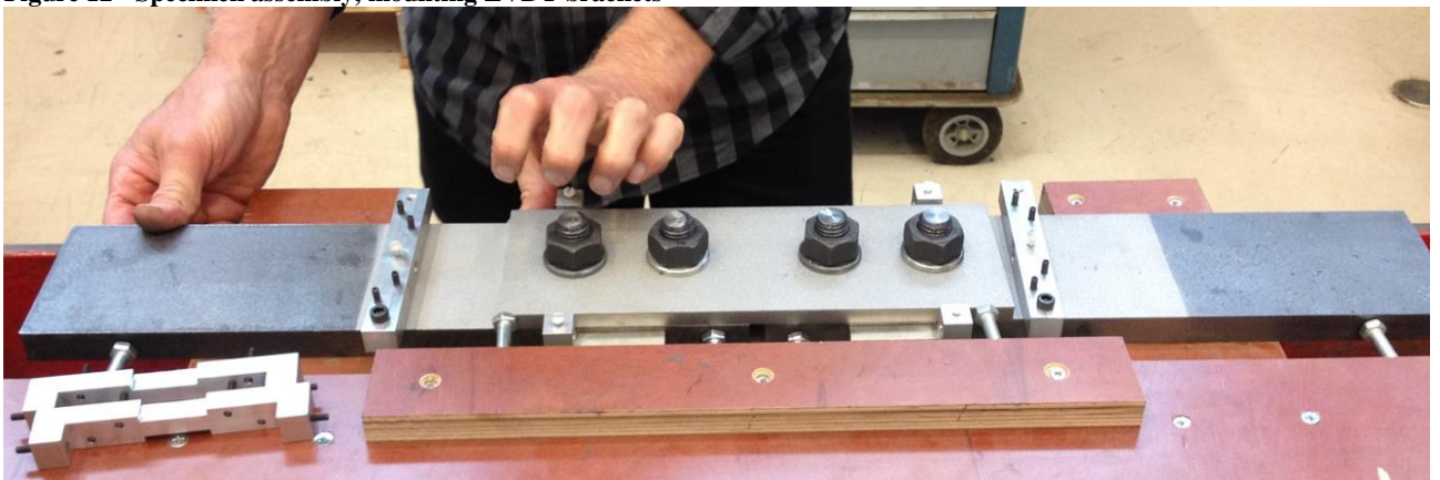
Figure 13 - Specimen assembly: alignment of centre / lap plates prior to pre-tensioning
