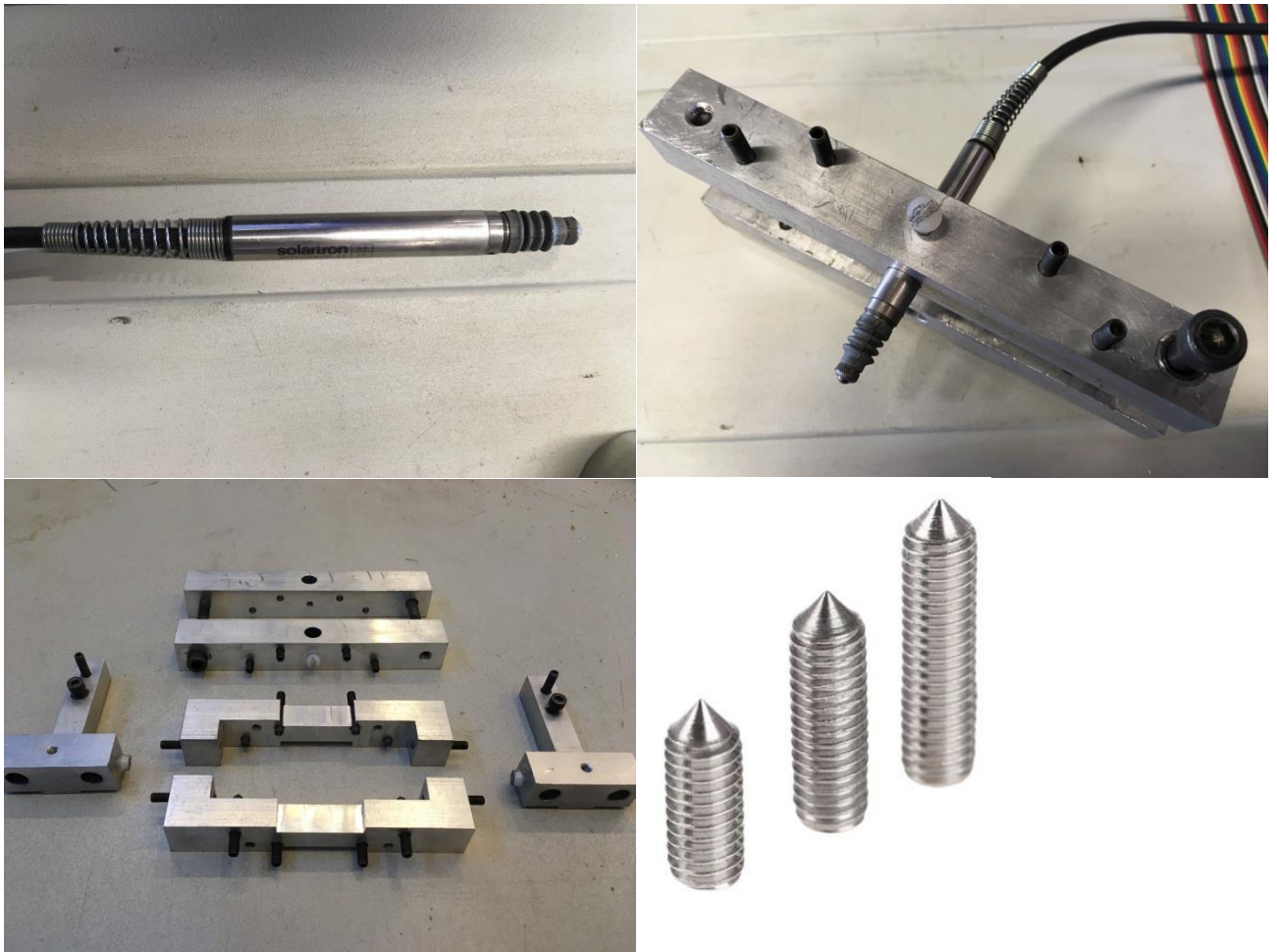
Figure 8 - Solartron AX 1.0 LVDT used for all slip measurements, various mounting brackets LVDT's. Lower right picture: Sharp tip allen screws were used to clamp/fixate mounting brackets to centre and lap plates
