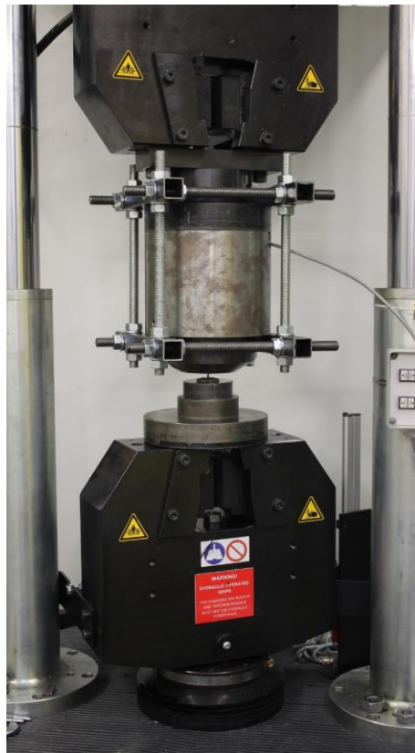
Figure 3 Test setup for compression test according to EN 14399-9
