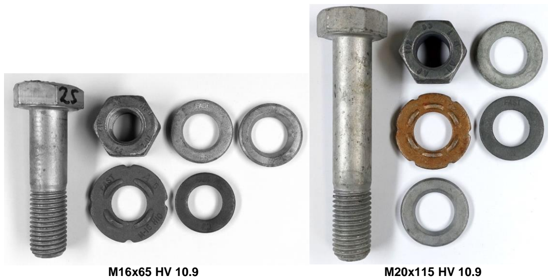
Figure 10 M16x65 HV 10.9 and M20x115 HV 10.9 bolting assemblies before testing including bolt face and nut face washers
