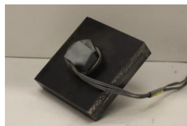
(f) One-bolt-specimen (75 mm x 75 mm plates)
