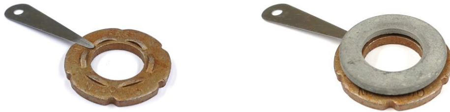
Figure 1 Use of a feeler gauge to check the gap
