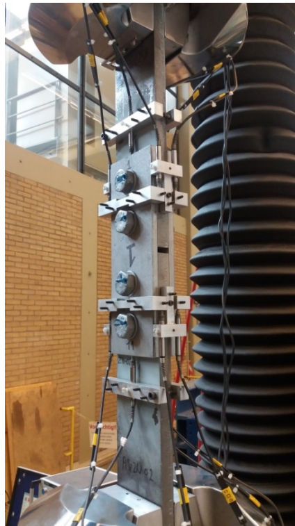
Figure 2.7: A specimen loading in the testing machine with 12 LVDT's
