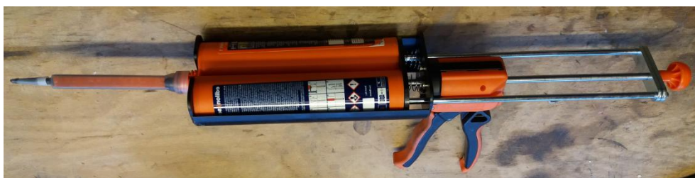
Figure 2.5: Special injection pistol only used for resin Edilon Dex-R2K
