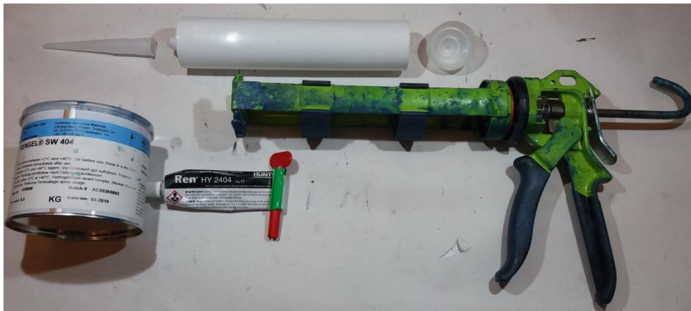
Figure 2.4: Injection pistol and equipment with resin Araldite
