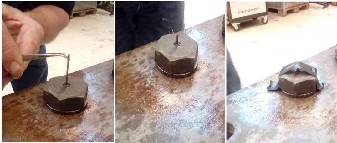
Figure 25 - Installation of the strain gauge in the hole filled with adhesive
