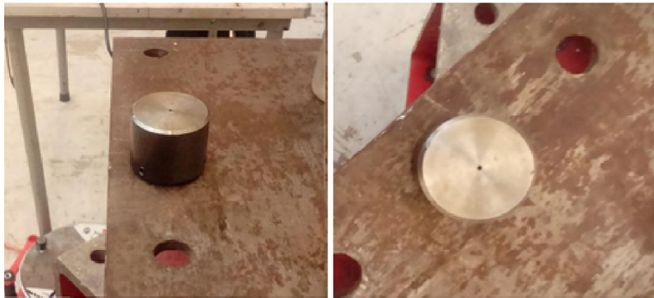
Figure 18 - Hexagonal steel die, designed to be fitted on the head of the bolt to (1) drill in the exact centre of the bolt and (2) ensure drilling parallel to the bolt axis
