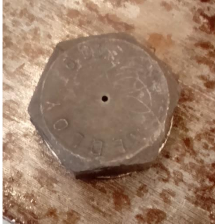
Figure 22 - Strain gauge hole drilled from the bolt head into the shank
