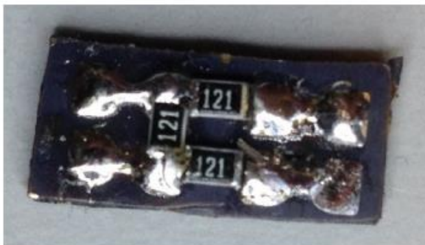
Detail picture of wire terminal on bolt heads. To minimise influence of temperature variation and cabling on the strain gauge measurements, a full Wheatstone bridge was integrated on each wire terminal. High precision micro resistors were used to create the bridge. Stevin report 6-18-03
