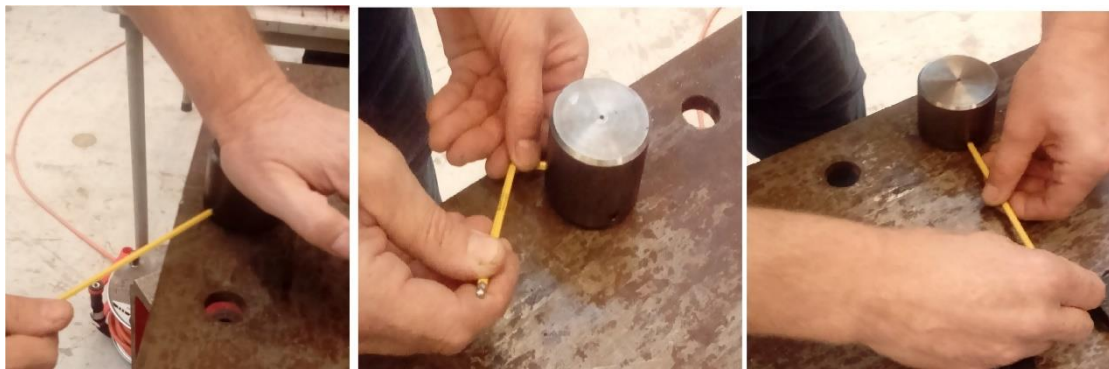
Figure 19 - Clamping of the hexagonal die on the head of the bolt
