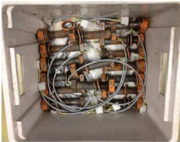
The 16 bolts that were removed from the connection were taken to the laboratory to verify linearity of the strain gauge signals and to determine the pretension that was present before untightening
