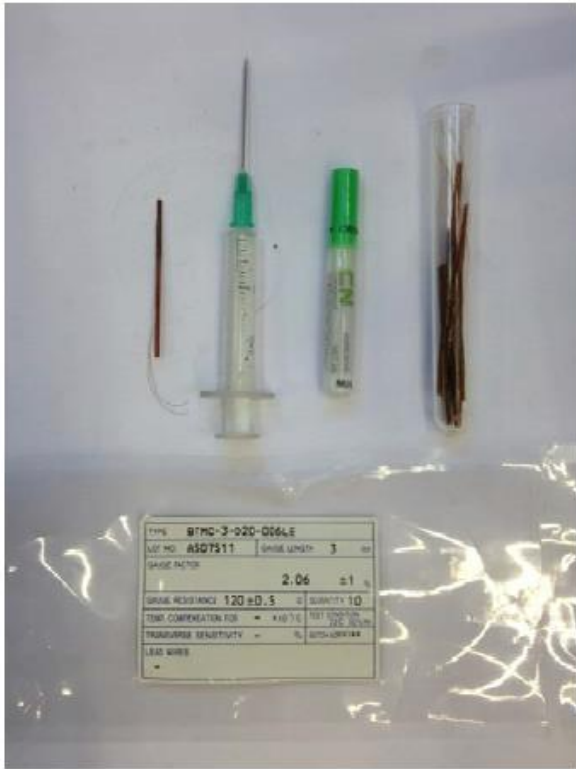
BTMC-3-D20-006LE strain gauges in combination with CN adhesive were used to instrument the bolts
