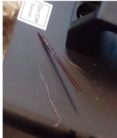
Figure 23 - BTMC strain gauge
