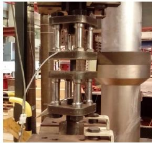
In the laboratory all bolts were loaded to determine the tensile force that corresponded to the strain measured during the in-situ untightening of the bolt. Linearity of all strain gauge signals was checked and confirmed. Finally the test setup was used to determine the tensile strength of the bolts.
