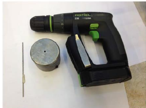
A hand held, battery driven machine was used to drill the holes. Special long VHSS steel drills were necessary to drill in the 10.9 material.
