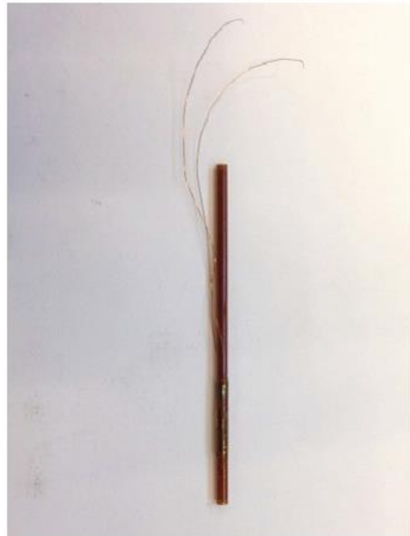
Strain gauge insertion pipe. The strain gauge itself is 3 mm long and is situated 10 mm from the lower end of the pipe.
