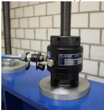
(b) tensiometer with the capacity of 600 kN
