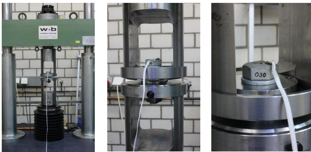
Figure 5 Calibration of instrumented bolts with strain gauge in the universal test machine (with a maximum load capacity of \pm 200 kN)
