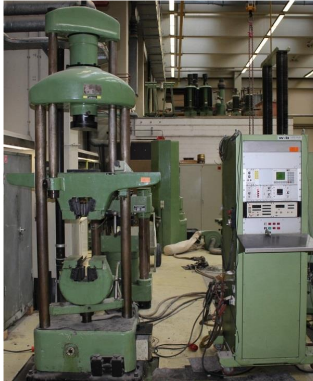
Figure 2 Servo-hydraulic universal testing machine (load capacity \pm 600 kN)
