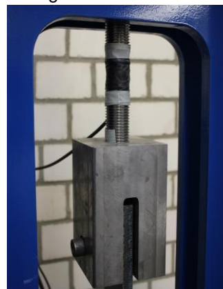
(c) instrumented threaded rod for measuring the load level
