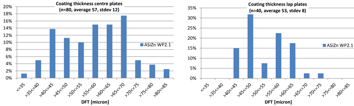
Figure 28 - Dry film thickness ASiZn plates
