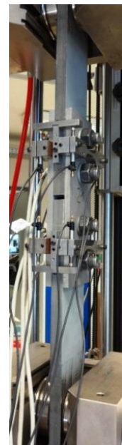
Figure 5: Result of long-term step test of zinc spray metallized (Zn-SM) specimen
