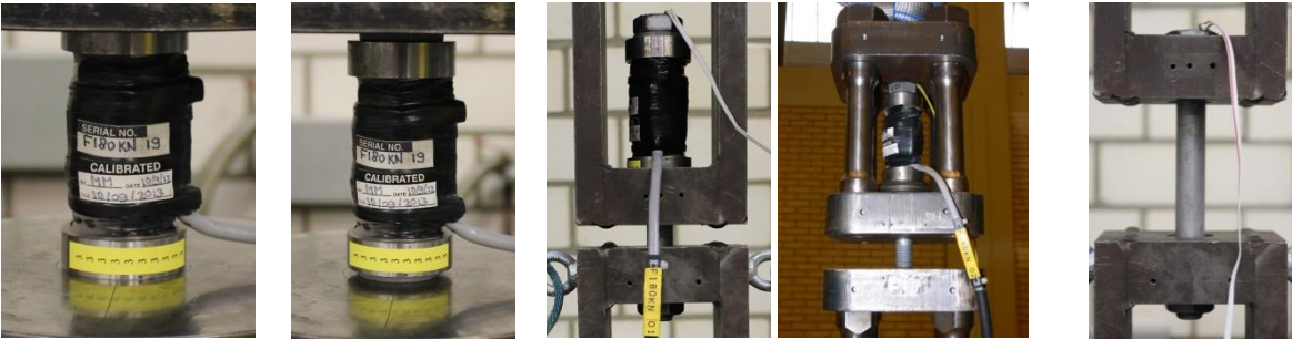
a) Compression test – load cell only b) Compression test – load cell with HV-washers c) Tension test – load cell with bolt calibrated at UDE (left) and TUD (right) d) Tension test – bolt only (UDE)
