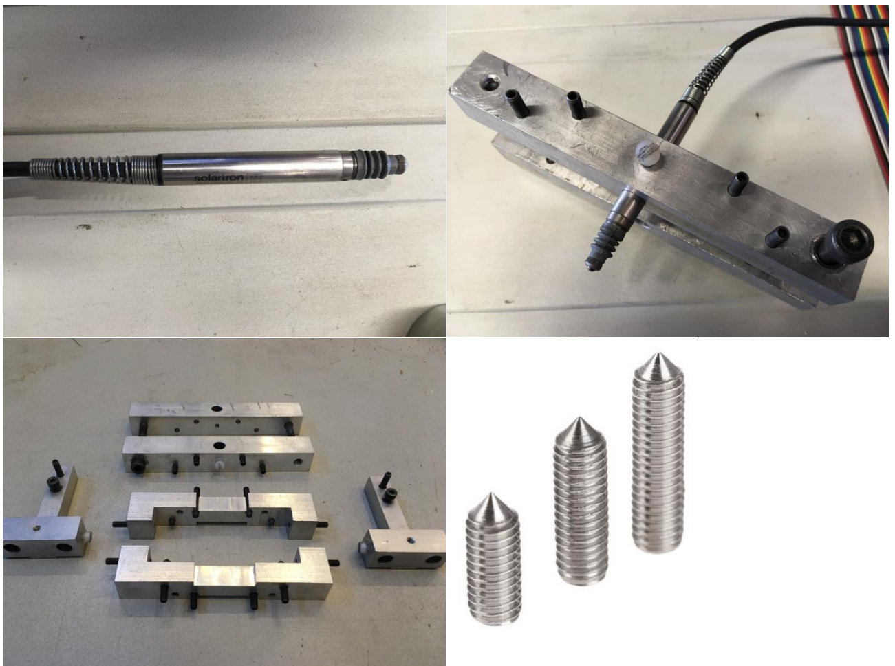
Figure 7 - Solartron AX 1.0 LVDT used for all slip measurements, various mounting brackets LVDT's. Lower right picture: Sharp tip allen screws were used to clamp/fixate mounting brackets to centre and lap plates
