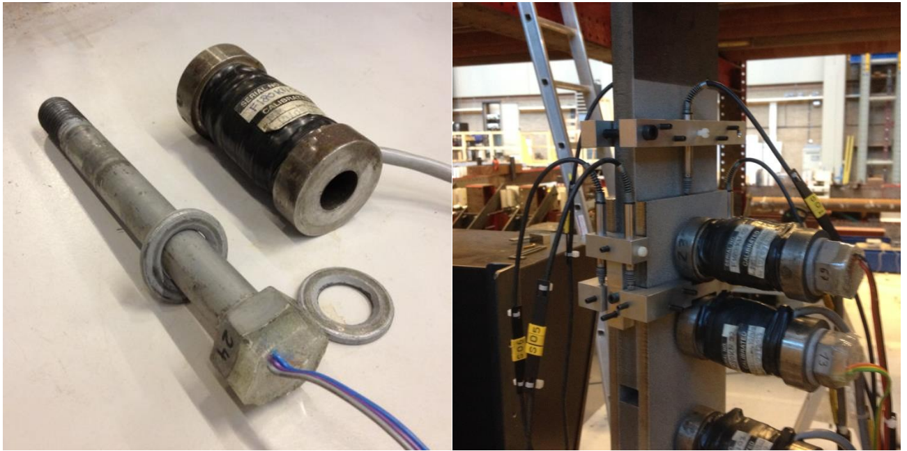
Figure 8 - Instrumented bolts M20,class10.9, TUD home made load cell (L=100mm); fully instrumented 'top connection' of a specimen
