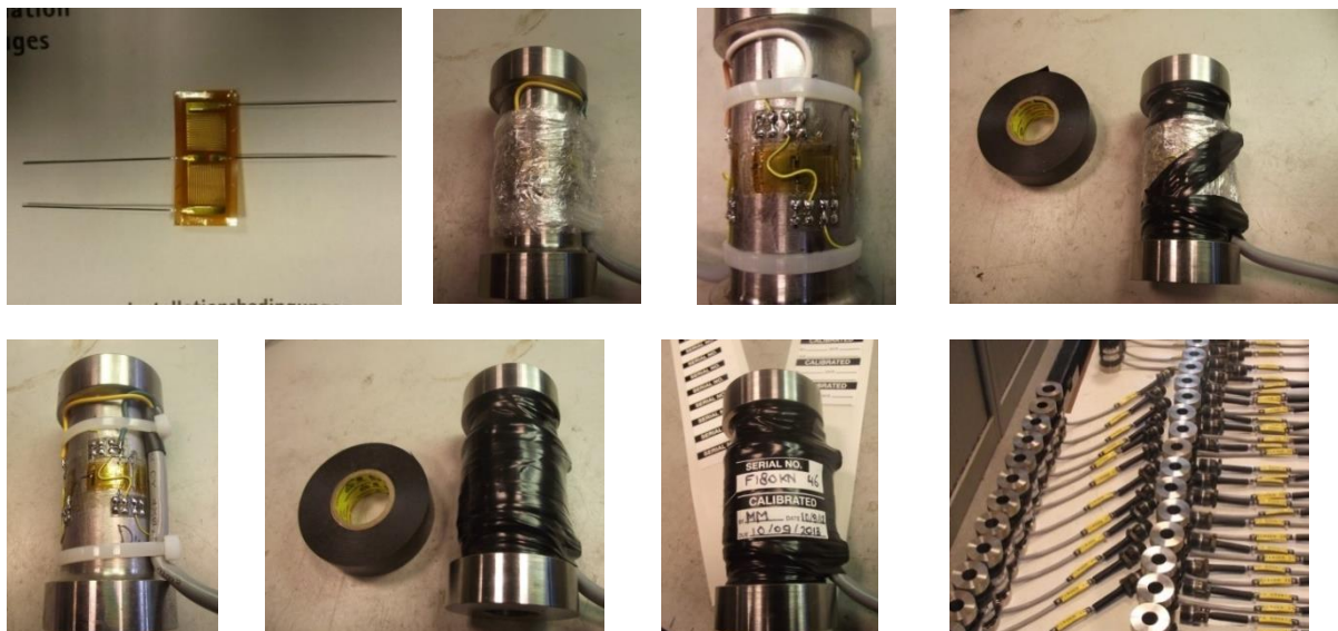
Figure 28 - Various phases of the production process of the load cells used in SIROCO (TUD)
