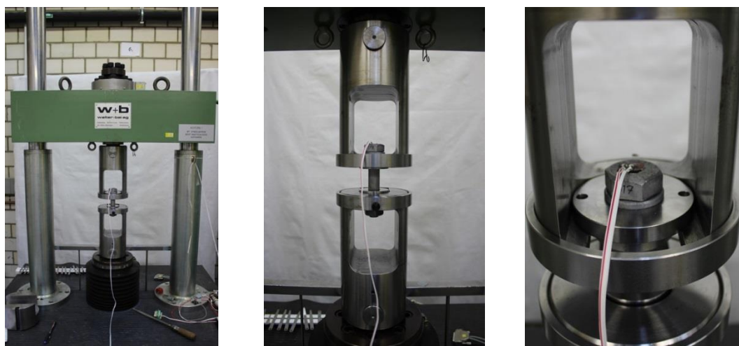
Figure 8: Calibration of instrumented bolts with strain gauge in a universal test machine (with a maximum load capacity of \pm 200 kN)
