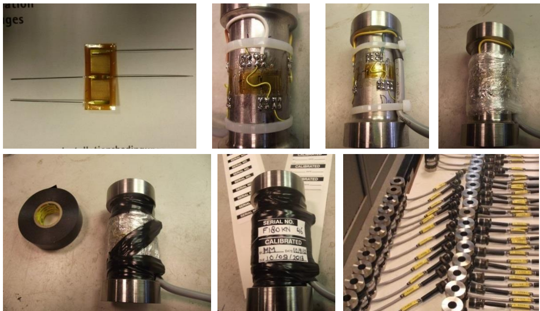
Figure 12: Various phases of the production process of the load cells used in SIROCO (TUD)
