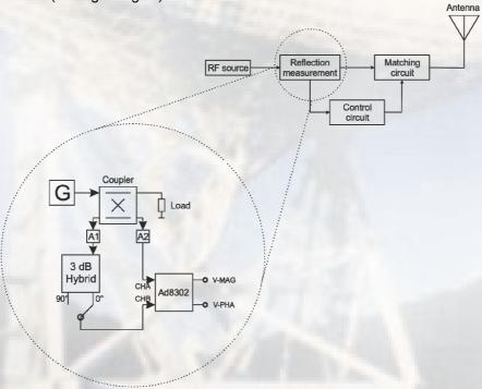
The task of the thesis is to build and investigate a reflectometer which measures the incident and reflected signals from a load. The measured vector reflection coefficient can be used to calculate the level of impedance mismatch and to control a matching circuit.
