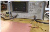
requires a piece of substrate to be cut from the large panel and is based on the evaluation of a simple microstrip line as a transmission line (testing the insertion phase) and as an open-ended transmission line resonator (testing the resonance frequency); the transmission line phase shift and resonance frequency can be compared to the theoretical values using well verified design formulas and the best-fit dielectric constant can be evaluated. The task in particular is to
