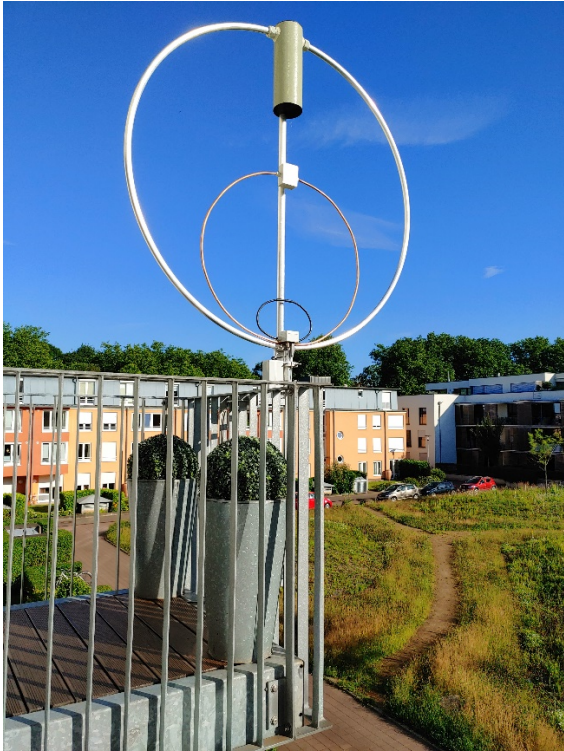
Fig.1 AMA82 - Antenna with second loop on our balcony.
