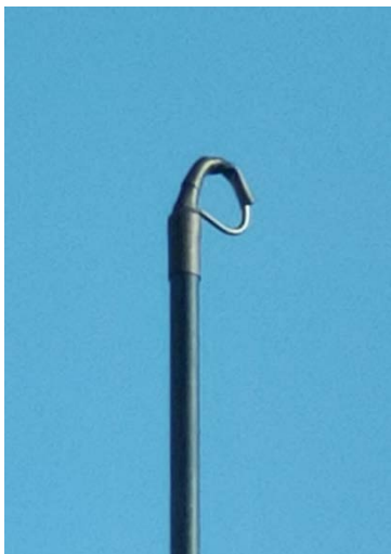
Figure 6 “Pig Tail” wires (seen with shrink tube sealing) at both ends of the dipole are used to tune the frequency of the dipole.
