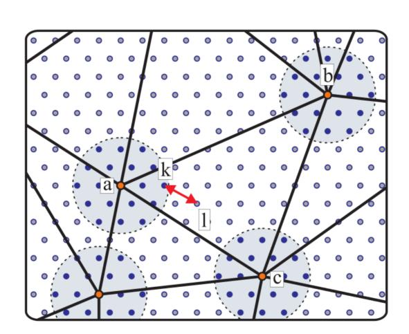
Crystal subject to FE-discretization (left) and with clusters around mesh-nodes for energy sampling (right). The method accounts for nonolocal atomic interactions everywhere.
