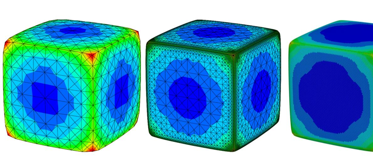
The contour plot of displacements  $u_r = \sqrt{(u_x^2 + u_y^2 + u_z^2)}$  [Å] reveals quantitative agreement (left and centre: adaptively refined FE meshes) of CQC-E results with (right) MS.
