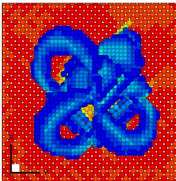
Fully atomistic resolution right below the indenter (left) for dislocation nucleation and microstructure evolution (centre and right), which is embedded in a halfspace (coarser finite element discretiziation) undergoing purely elastic deformation.
