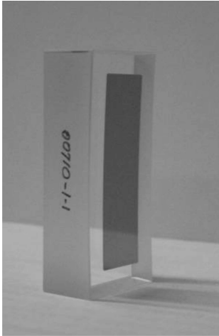
Figure 3.12: Photography of the toroidal Ge mirror attached to the glass substrate. Source: Shymanovich [27] .
