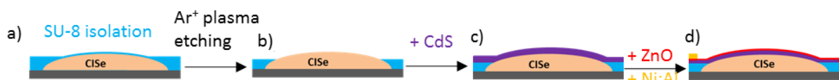
Figure 2: Scheme of electrical isolation process of the micro-absorber, consisting of spin-coating of SU-8 (a), \text{Ar}^+ plasma etching (b), CdS buffer layer deposition (c), and ZnO front contact deposition (d).
